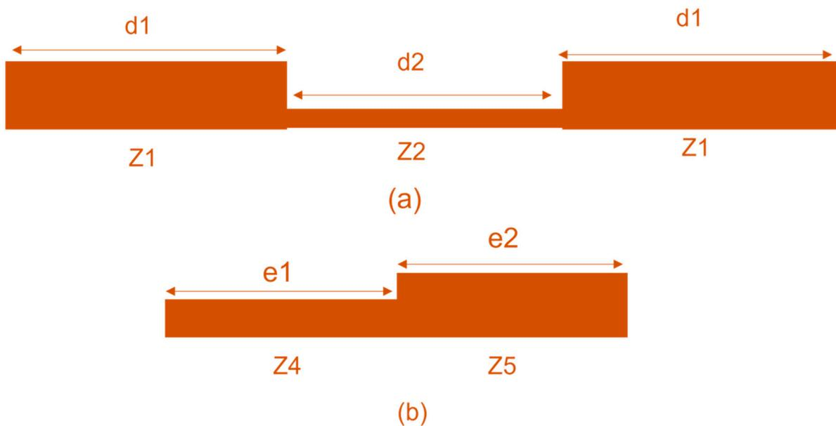
Figure 3. SIR varieties: (a) SSIR type; (b) ASIR type.
