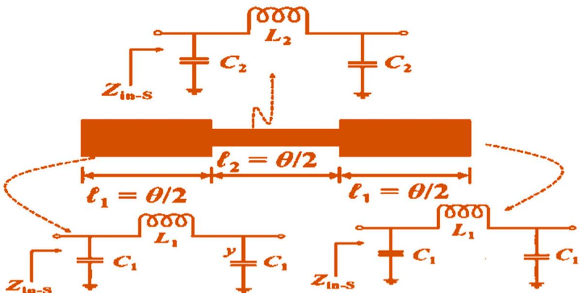
Figure 5. The lumped element circuit equivalent for SIR under operating resonant frequency.
