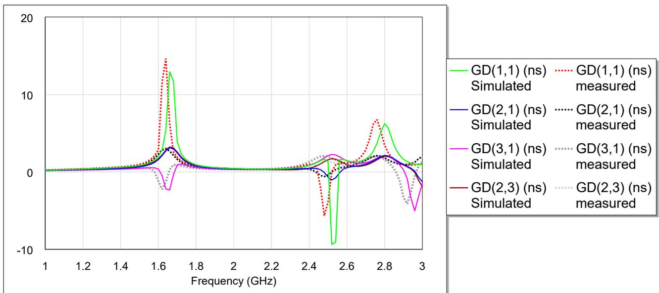
Figure 14. Comparison between simulations and measurements in terms of GD.
