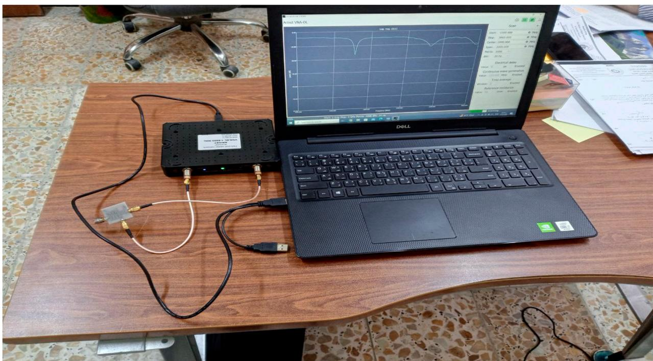
Figure 12. The setup for measurement based on the selected S-parameter (S11) with 50-ohm termination.
