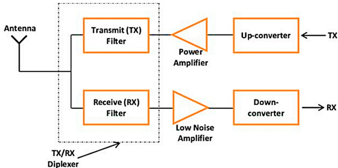
Figure 1. Diplexer in RF front end.
