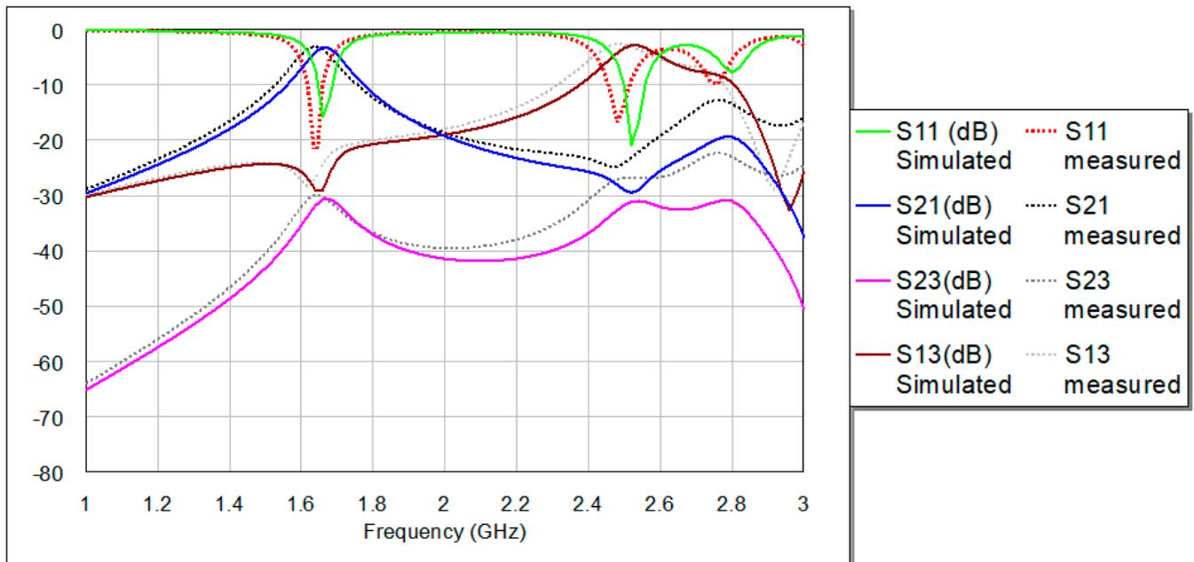
Figure 13. Comparison between simulations and measurements in terms of S-parameters.
