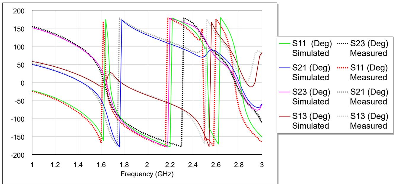
Figure 15. Comparison between simulations and measurements in terms of phase.
