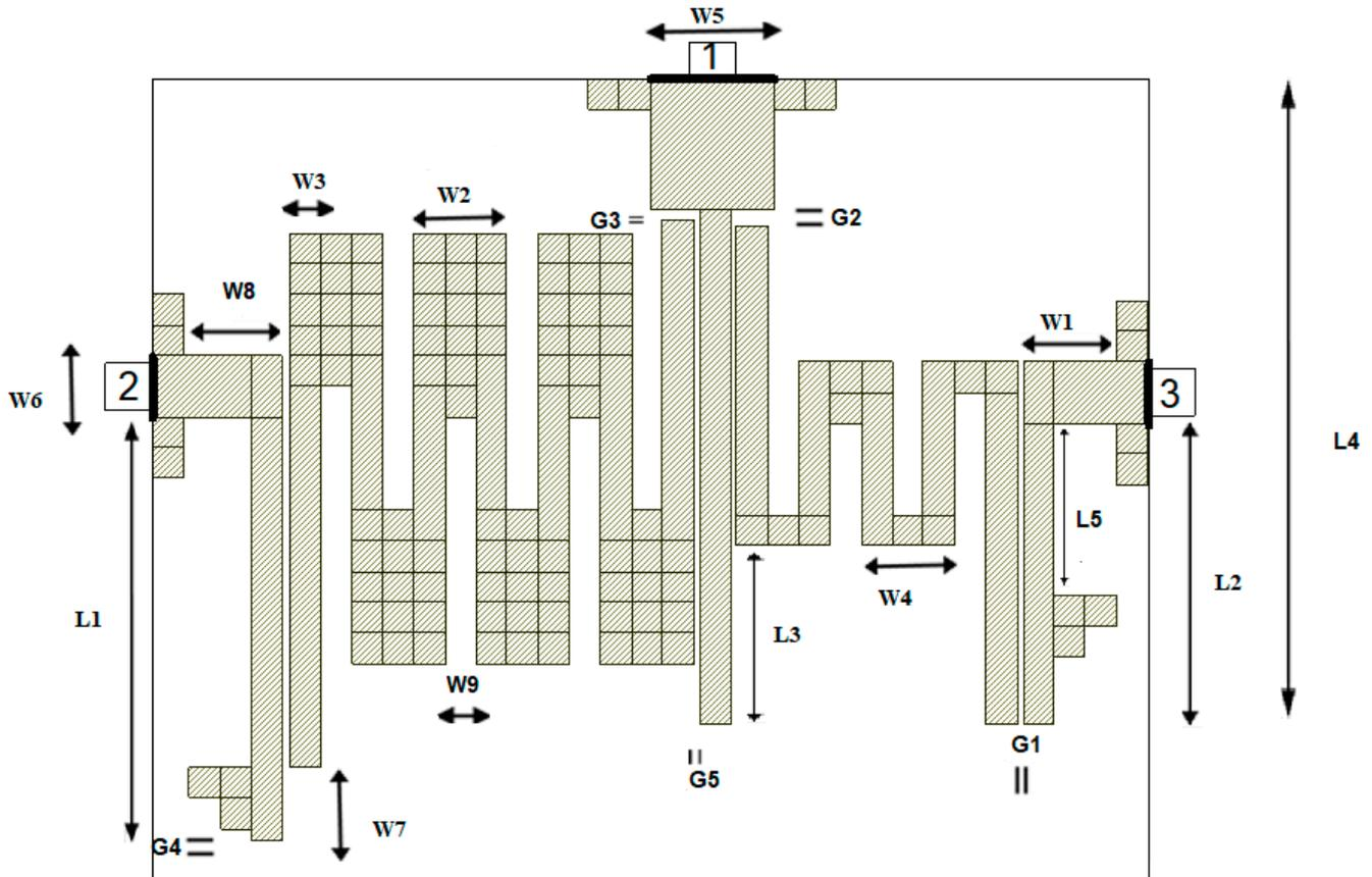
**Figure 7.** Suggested Diplexer Topology.  $W1 = 3.01$ ,  $W2 = 2.98$ ,  $W3 = 1$ ,  $W4 = 2.98$ ,  $W5 = 4$ ,  $W6 = 2$ ,  $W7 = 2.4$ ,  $W8 = 3.2$ ,  $W9 = 1$ ,  $L1 = 13.8$ ,  $L2 = 9.8$ ,  $L3 = 5.8$ ,  $L4 = 21$ ,  $L5 = 5.6$ ,  $G1 = 0.19$ ,  $G2 = 0.6$ ,  $G3 = 0.4$ ,  $G4 = 0.4$ ,  $G5 = 0.2$ . The diplexer dimensions (in mm units).
