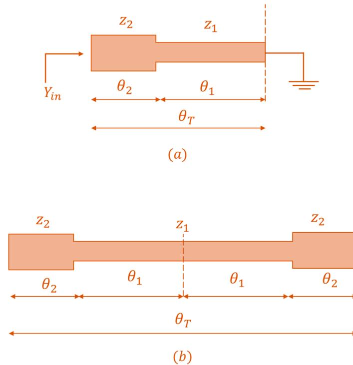
Figure 2. (a) The quarter-wavelength type, and (b) the half-wavelength type for the SIR variants.
