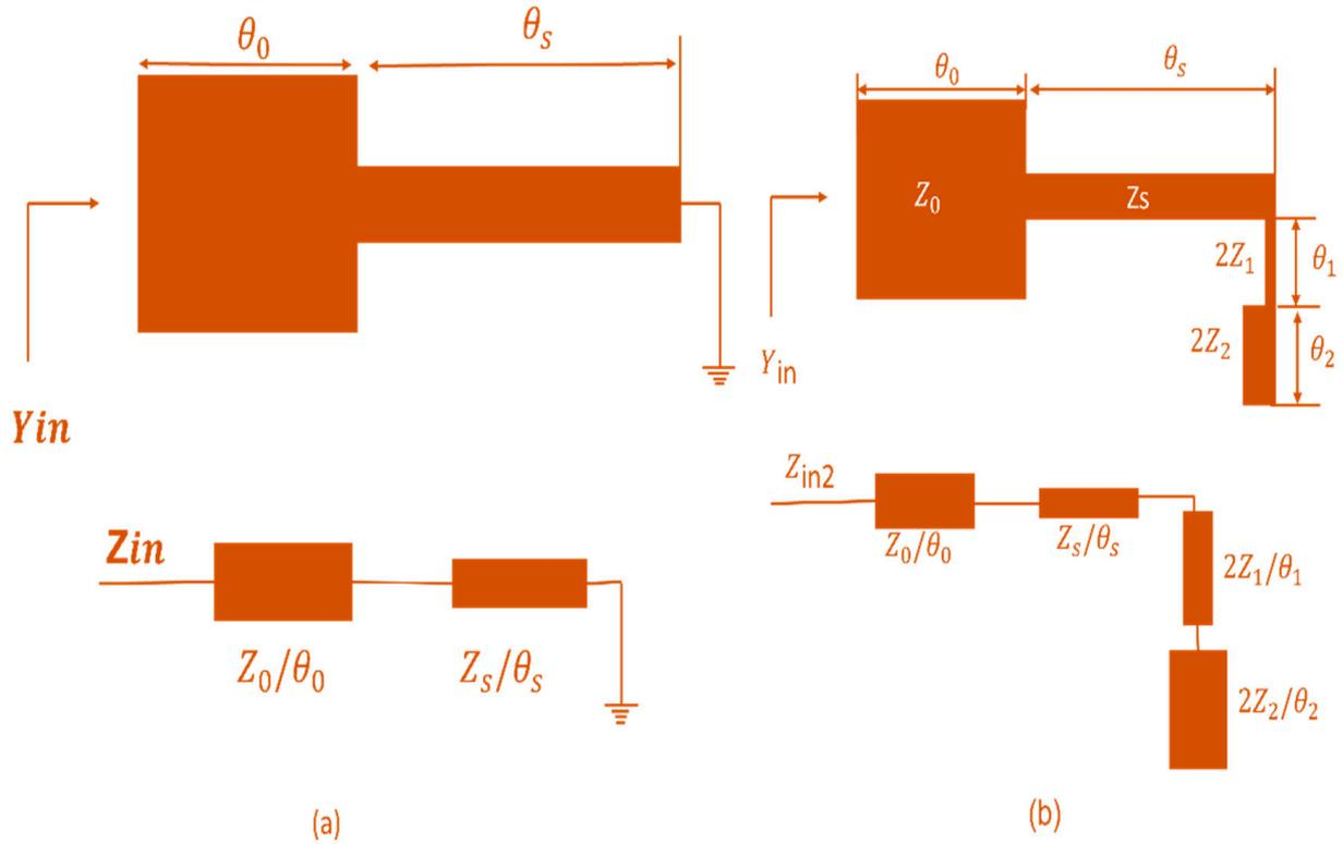
Figure 4. (a) Odd and (b) even resonance representations for SIR.
