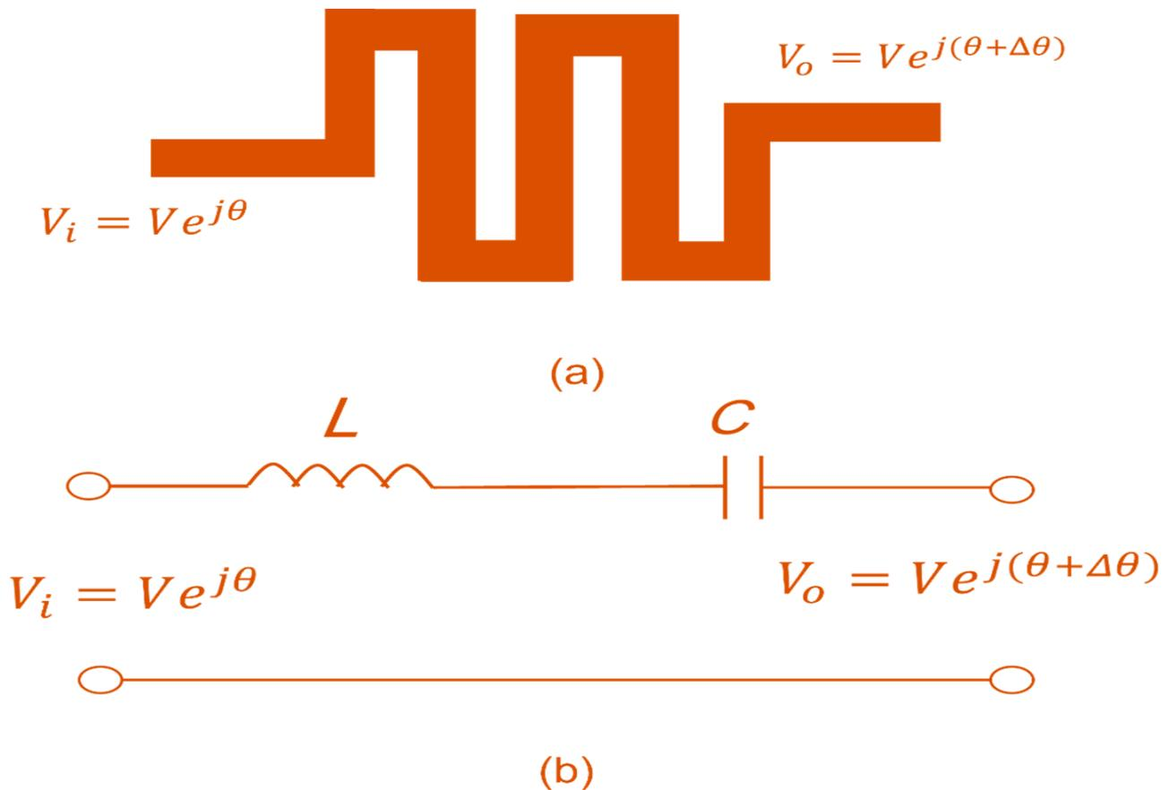
**Figure 6.** (a) The typical structure of a meander resonator, and (b) its equivalent lumped element circuit.
