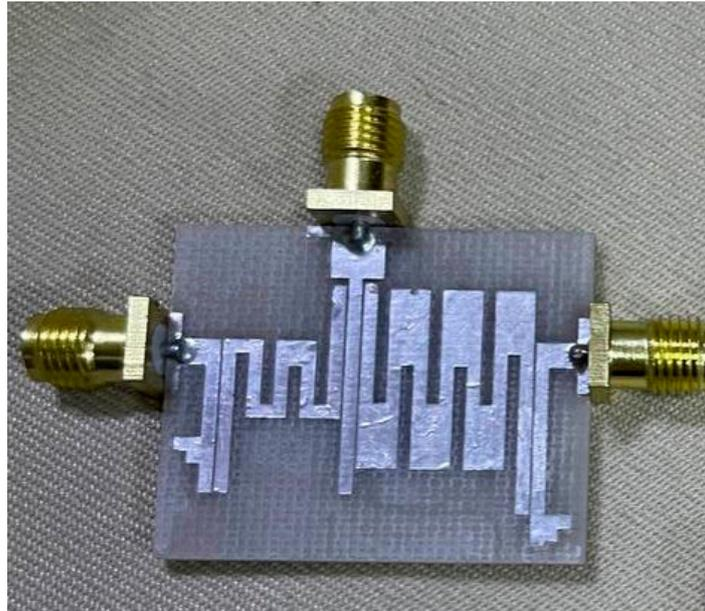
Figure 11. The fabricated diplexer prototype.
