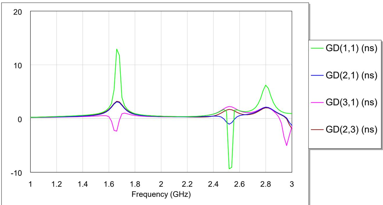
Figure 9. The Simulation GD for the designed microstrip diplexer.
