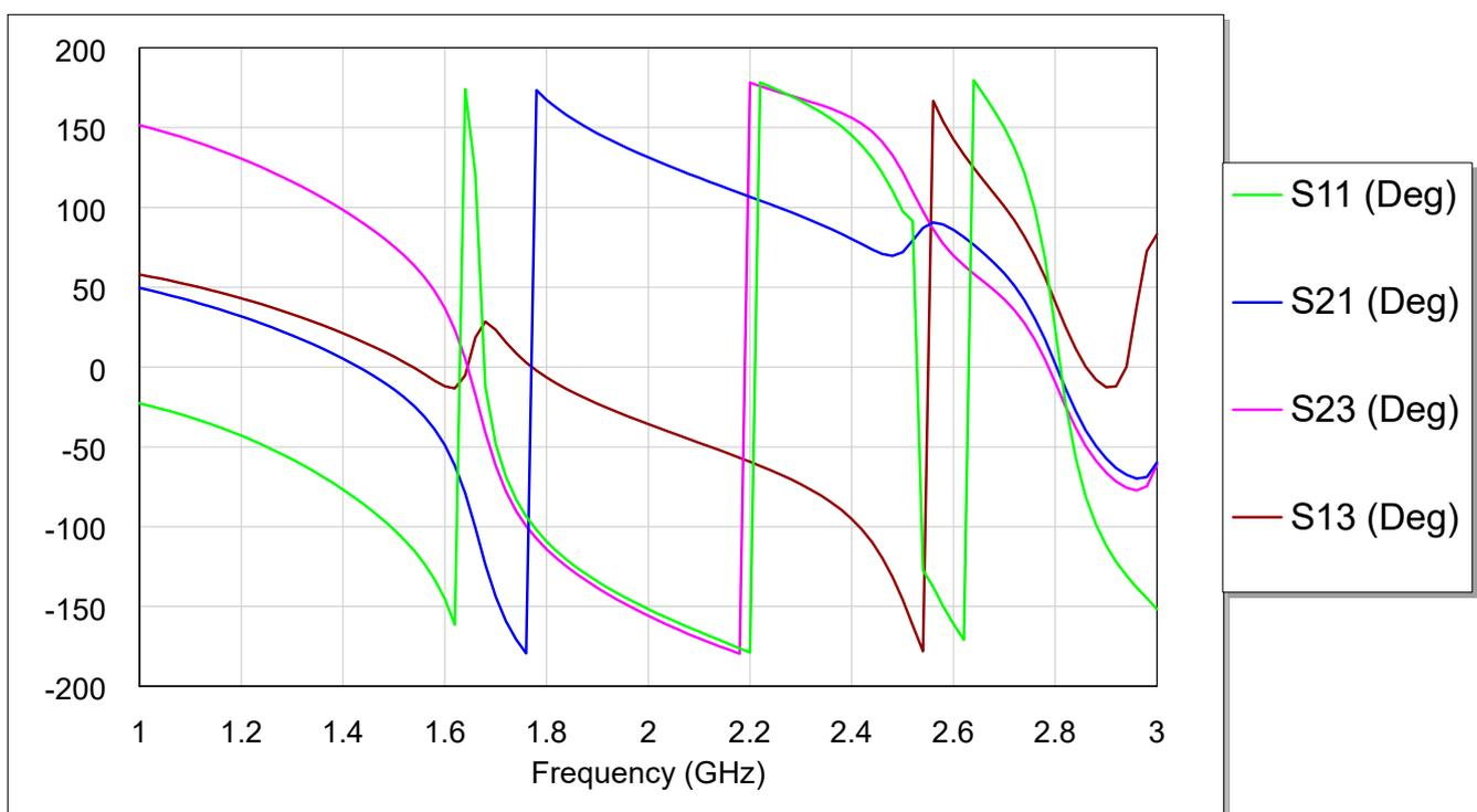
**Figure 10.** Phase response for the projected diplexer for each S-parameter.
