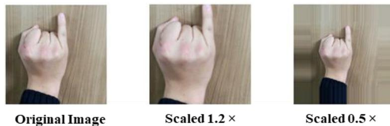
Figure 3. Image Scaling Illustration.
