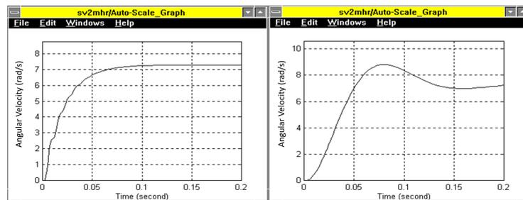
**Figure 8.** Rotary hydraulic actuator with a servo valve simulation results with inertial correction of the servo valve, the graph on the left is with first-order inertial correction included with  $T_i = 0.02$  sec the overshoot is reduced, but the response time is increased, and the graph on the right is with second-order inertial correction with  $T_{i2} = 0.0005$  s and  $T_{i1} = 0.02$  s, a large response time is introduced and the transient time is increased but operation is stable.
