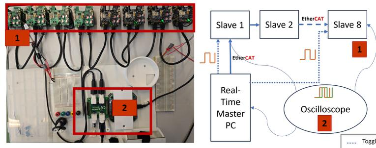
**Figure 17.** Conducted test for evaluating network latency.
