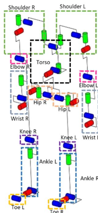
Figure 11. Distribution of the joint controllers of HYDROiD upon mechanism.
