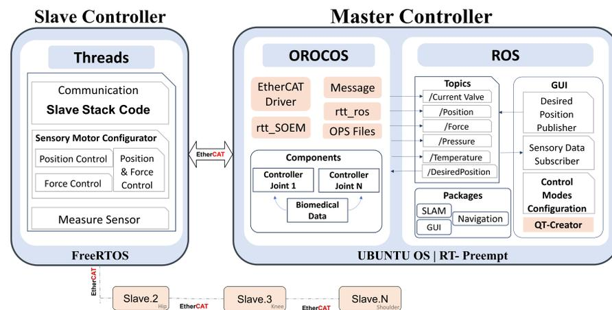
Figure 13. Developed control architecture for HYDROiD's control.
