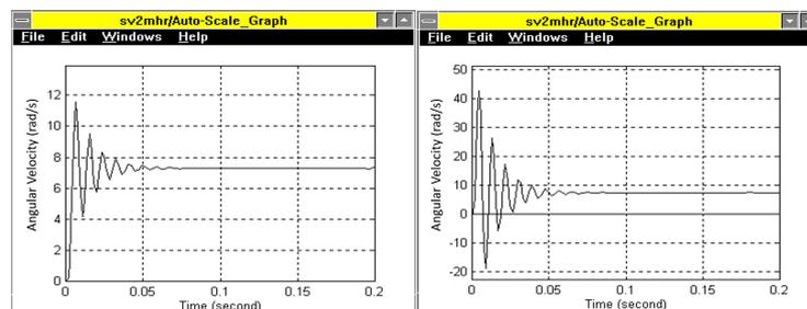
**Figure 7.** Rotary hydraulic actuator with a servo valve simulation results with anticipation and inertial correction of the servo valve, the graph on the left is with inertial correction with  $T_d = 0.0001$  and  $T_i = 0.001$ , the overshoot increased and the response time decreased, and the graph on the right is with anticipation correction with  $T_d = 0.01$  and  $T_i = 0.001$  the overshoot increased, the response time decreased and the transient time increased.
