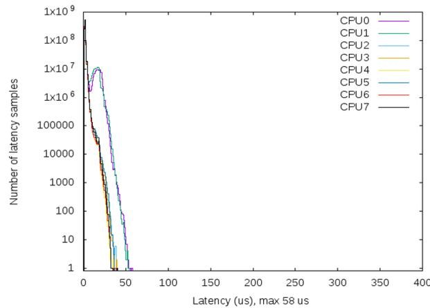
Figure 20. Latency of real-time Ubuntu kernel.
