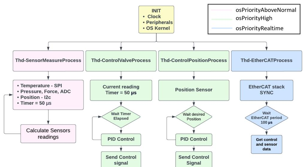
Figure 12. Developed tasks for the joint controller.
