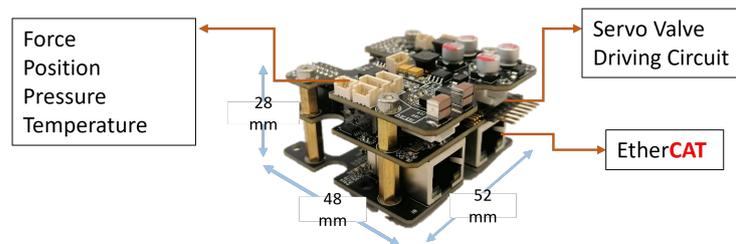
Figure 10. Developed electronic board at the joint level.
