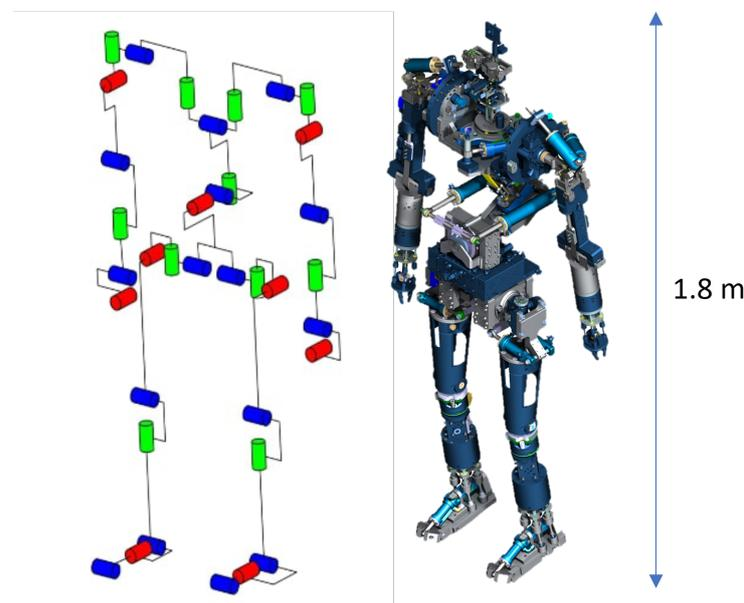
**Figure 2.** HYDROiD's kinematic structure.
