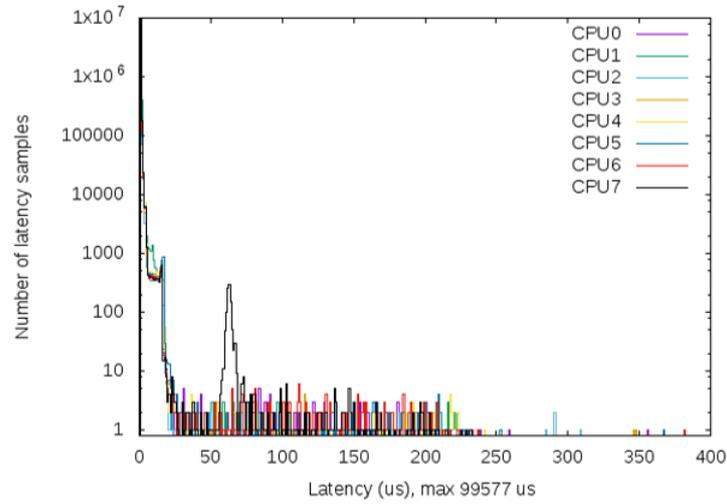
Figure 19. Latency of standard Ubuntu kernel.
