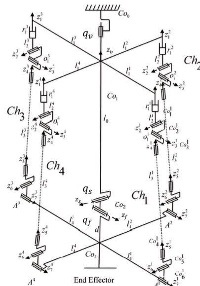
Figure 4. Kinematic structure of HYDROiD’s ankle mechanism.
