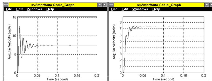
**Figure 6.** Rotary hydraulic actuator with a servo valve simulation results, the graph on the left is without the servo valve correction there is an overshoot, the graph on the right is with the servo valve correction included with  $T = 0.006$  s, the overshoot is reduced and the response time is increased.
