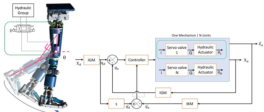
Figure 3. Control of one mechanism in HYDROiD.
