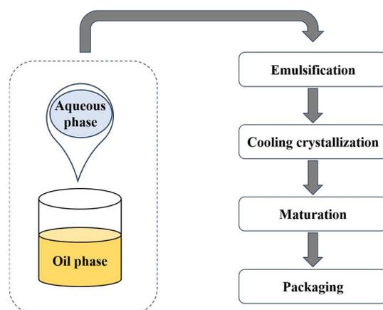
Figure 1. Margarine production process.
