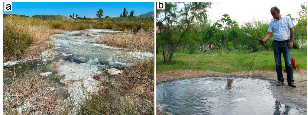
Figure 6. White Water (Uji Bardhe) thermal springs at the Makaresh karst massif. (a) The main spring; (b) measuring the water conductivity at the free-flowing Zheji borehole (photo Eftimi R.).
