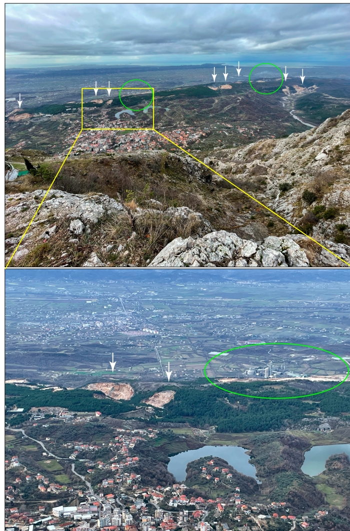
Figure 9. Panoramic views of the Makaresh area: the picture above shows the many quarries (white arrows) and the location of the two cement factories (green circles) located at the top of the karst plateau; below, magnification of the area delimited by the yellow rectangle.
