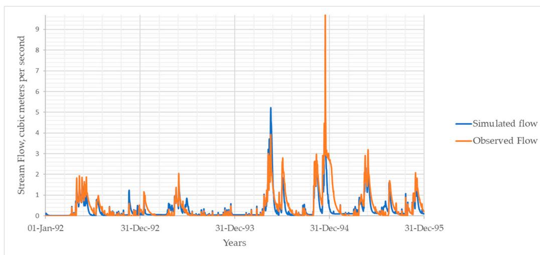
**Figure 6.** Daily observed and simulated discharge for entire validation period (1992–1995).
