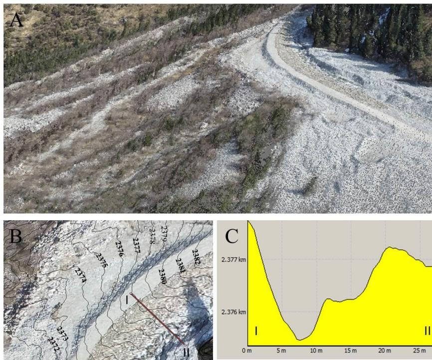
Figure S4. A. 3D model of Aksay cone and dam B. Cross-section (I-II) in the top part of protective dam C. Cross-section (I-II) created in Agisoft
