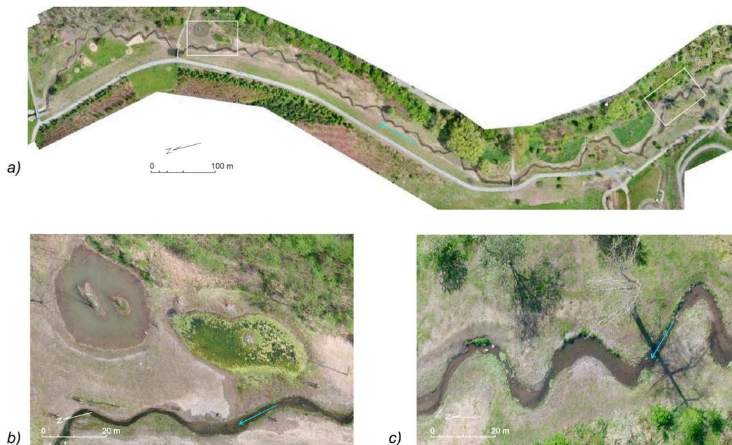
**Figure 4.** Orthoimagery of Hostavicky brook from June 2016. (a) Overview of the study site, (b) detailed view of the newly built ponds, (c) detailed view of the newly designed meanders of the stream.
