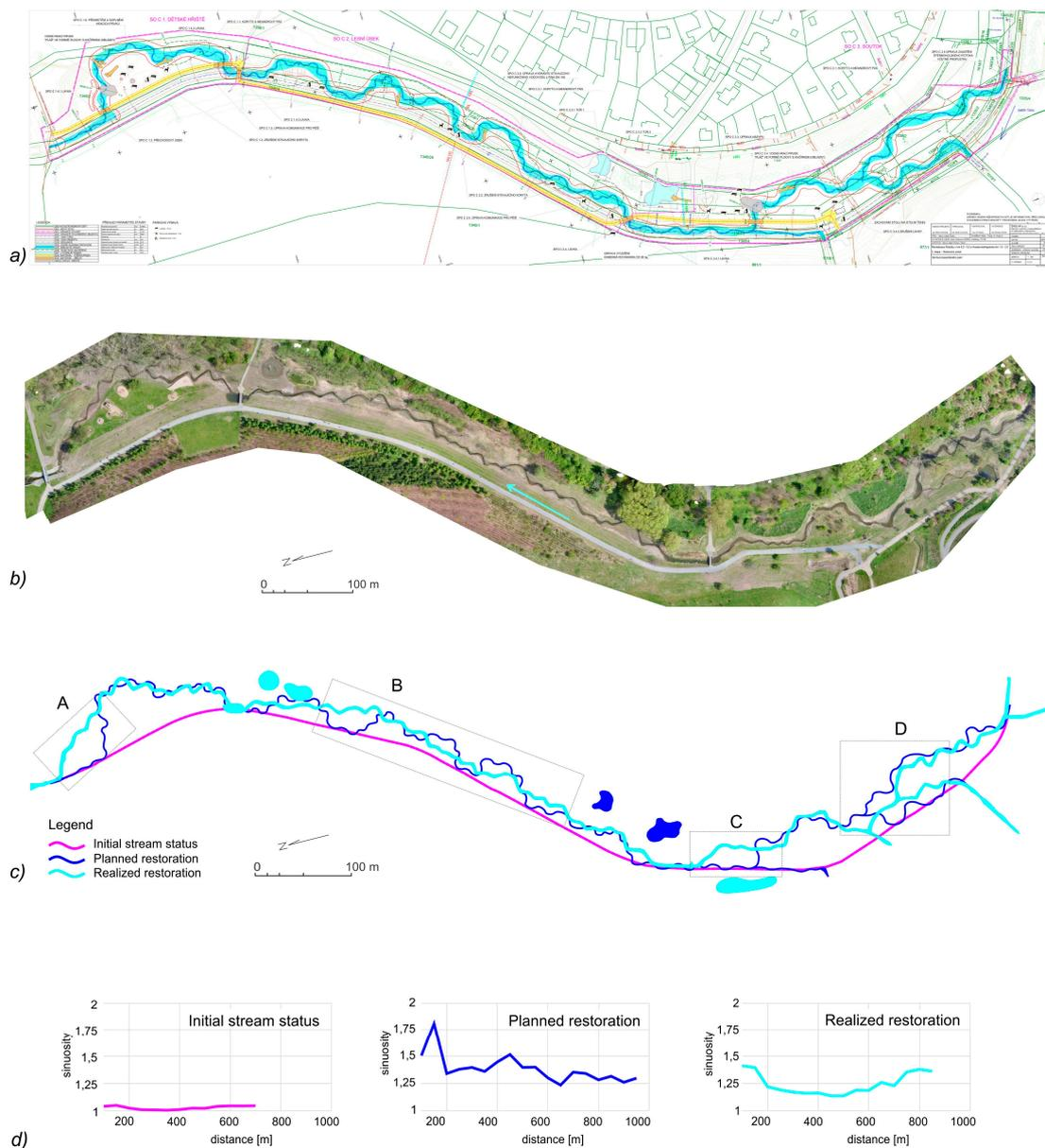
**Figure 7.** Fit of the resulting stream restoration to the plan. (a) Initial status and plan of the restoration, (b) newly shaped channel, six months after restoration, (c) identification of stream segments where the restoration has deviated from the plan, and (d) changes in stream length and sinuosity.
