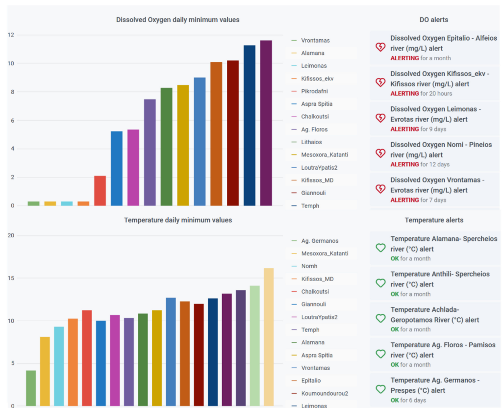
Figure 11. Bar charts of the minimum daily values for the physicochemical parameters of water dissolved oxygen (DO) and water temperature (T) measured from the monitoring network of stations (along with the active alerts for every station and parameter, as presented in the HCMR central visualization platform).
