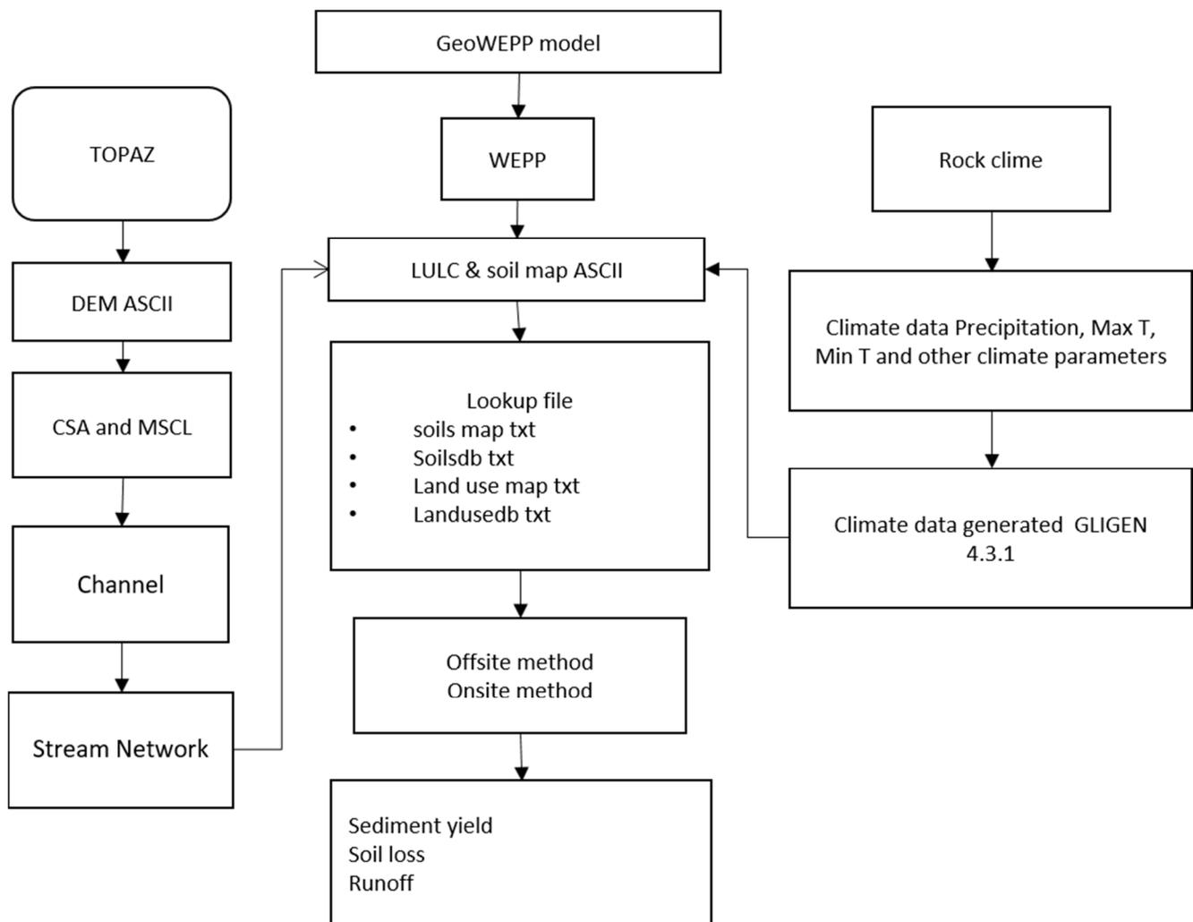
**Figure 2.** Methodology flow chart and descriptions of the CSA-Critical Source Area, MSCL-Minimum Source Channel Length, and CLIGEN-Climate Generator.
