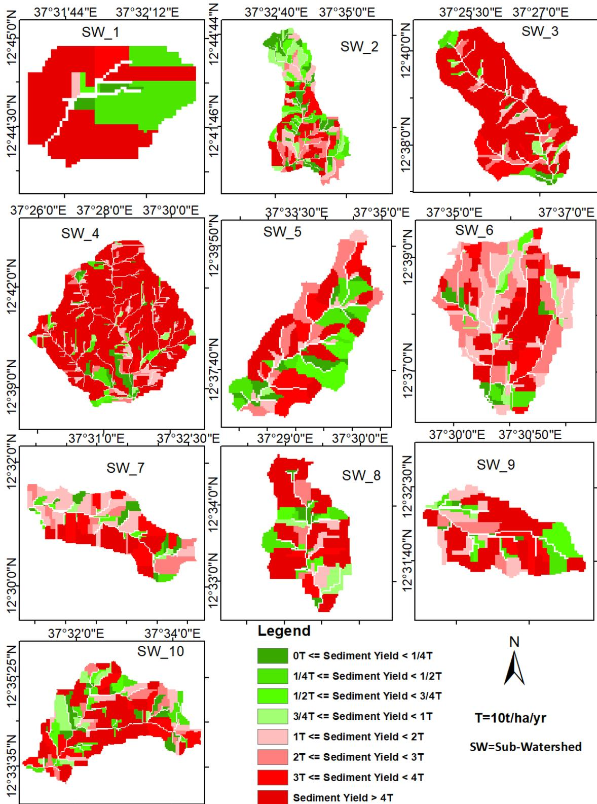
Figure 10. Offsite (watershed) method of the GeoWEPP model simulation for ten selected sub-watersheds (sediment yield map) relative to tolerable (T) value.
