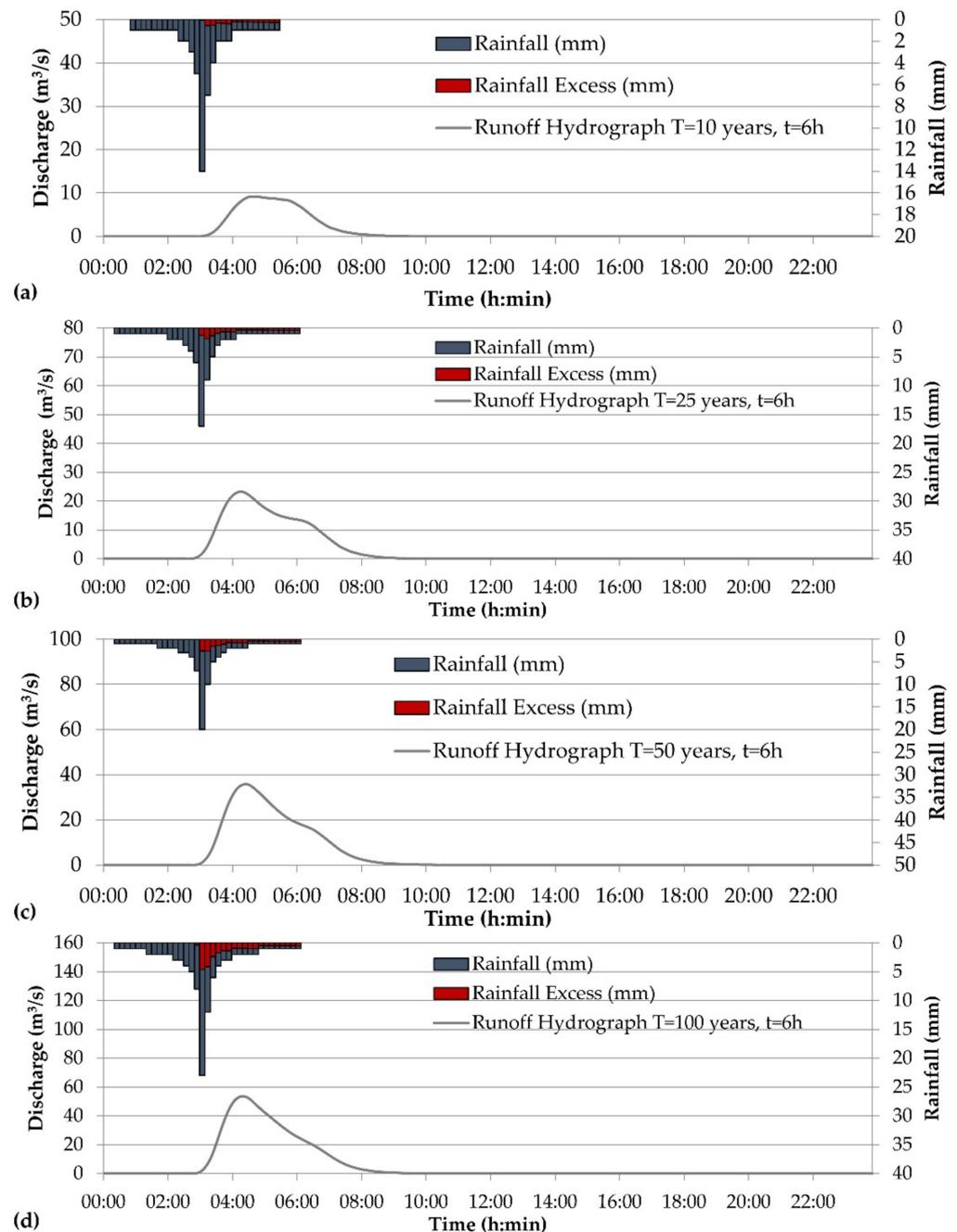
**Figure 4.** Hydrologic simulations for rainfall duration of 6 h and return periods of (a) 10 years, (b) 25 years, (c) 50 years and (d) 100 years.
