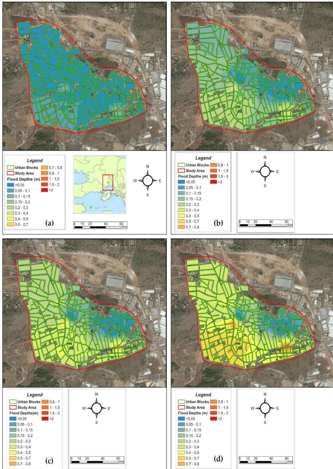
**Figure 5.** Flood inundation depths for rainfall duration of 6 h and return periods of (a) 10 years, (b) 25 years, (c) 50 year and (d) 100 years.
