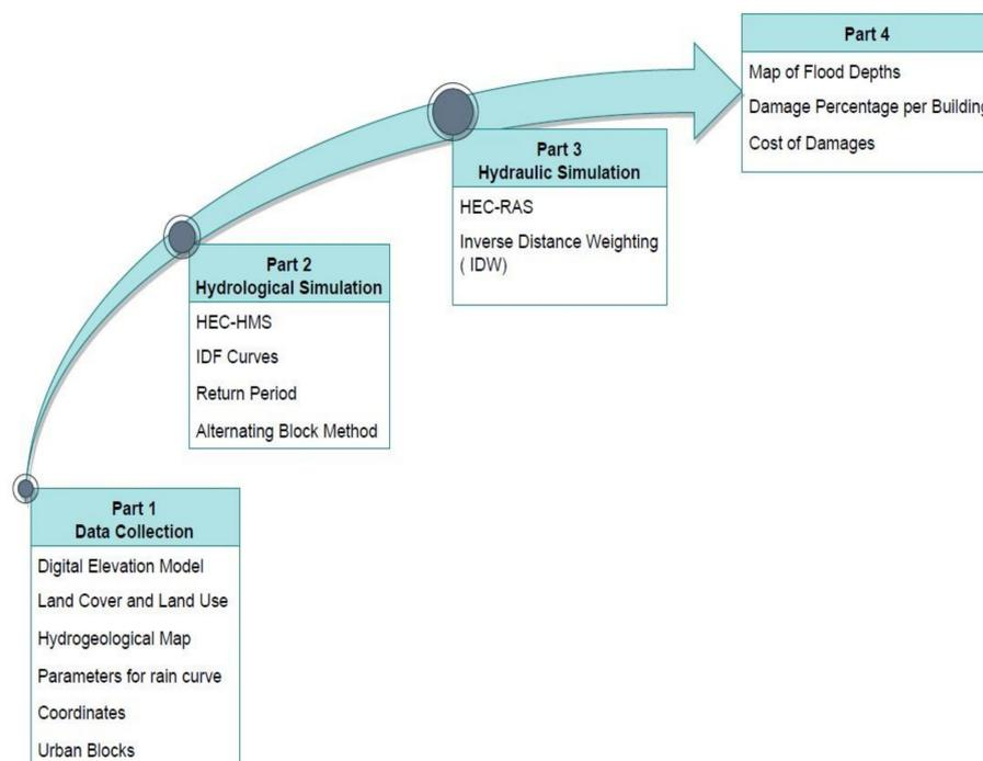
**Figure 1.** Flow chart of the proposed data-driven tool for flood risk assessment.
