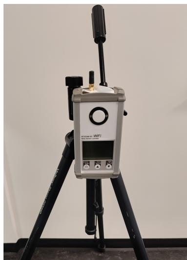
**Figure 11.** Measurement setup of the Gigahertz BTS256-EF Spectrometer on a tripod.
