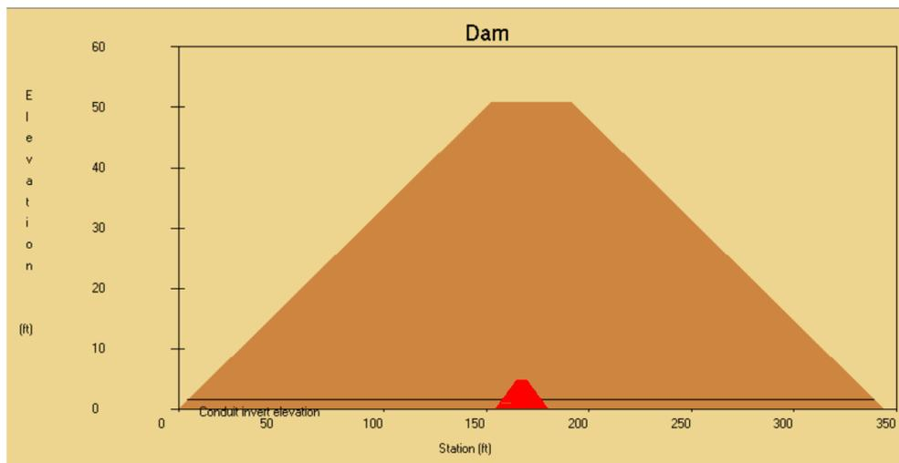
**Figure 1.** Comparison of the side profiles of the Big Bay (brown) and P1 (red) dams.
