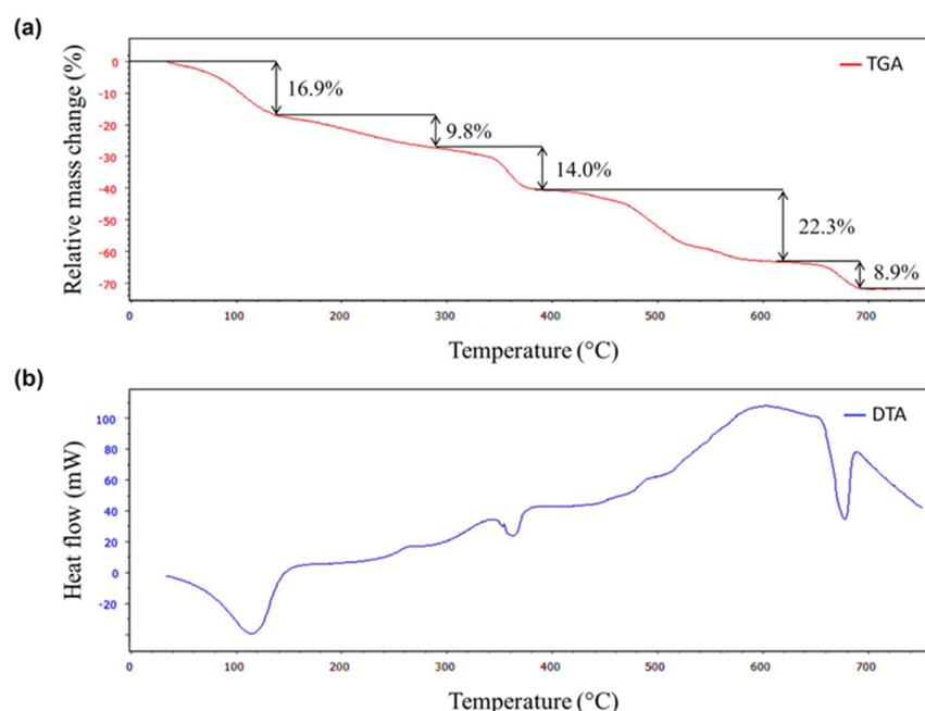
**Figure 4.** (a) TGA and (b) DTA profile of MIL-88B(Fe).
