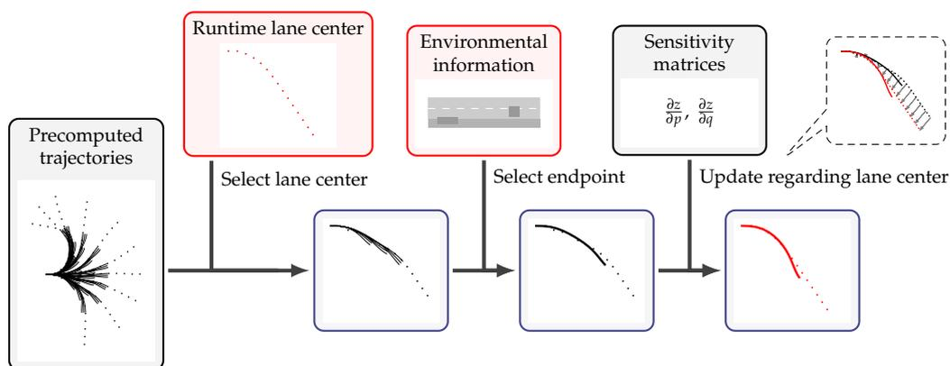
**Figure 5.** Process of the trajectory computation at runtime. Gray boxes indicate inputs from the precomputation phase; red boxes indicate inputs from sensor fusion.
