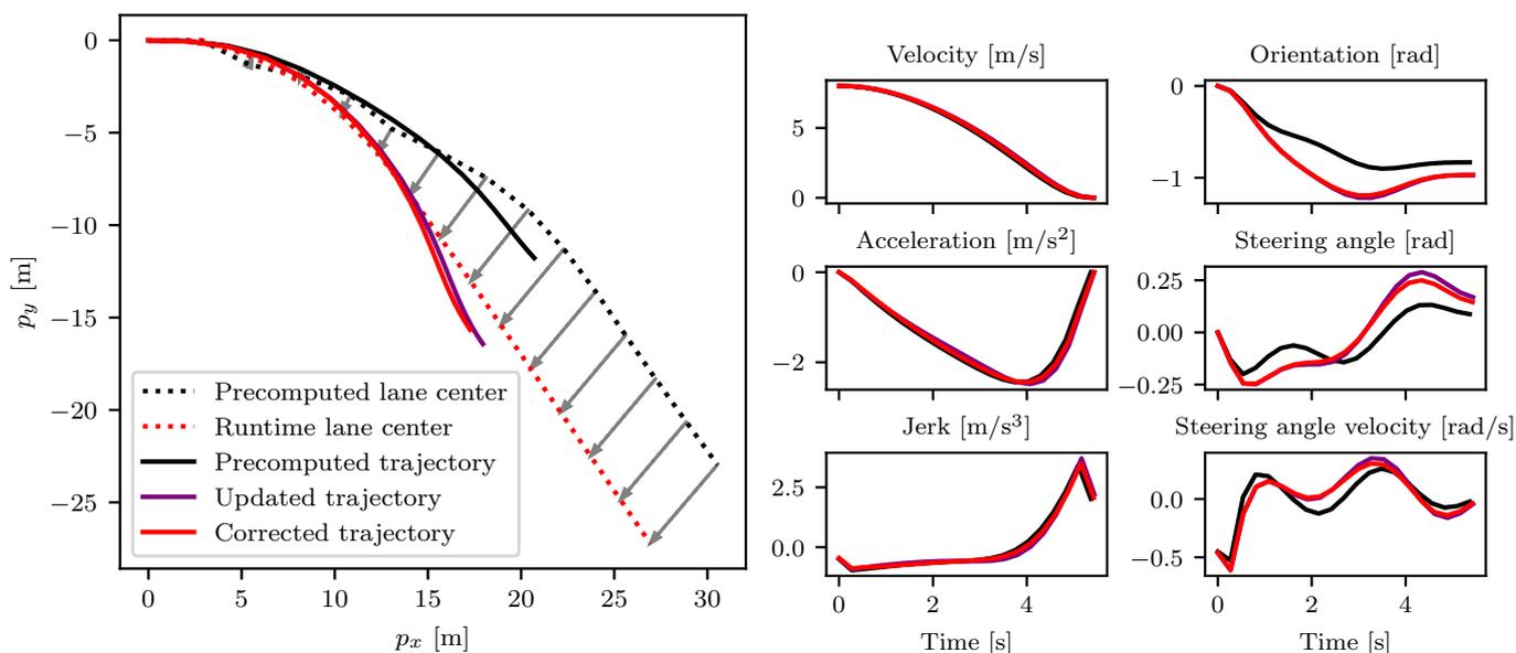
**Figure 7.** Exemplary trajectory during the process of trajectory computation. The selected pre-computed trajectory, the trajectory after the parametric sensitivity update with respect to changes in the lane center coordinates, and the trajectory after feasibility correction are displayed. On the left, the position in Cartesian coordinates is presented; on the right the other states and controls are presented.
