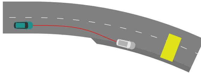
**Figure 1.** Exemplary scenario that may require a stopping maneuver. The yellow obstacle obstructs the street. The turquoise car depicts the initial position; the gray car depicts the final position. The computed safe stop trajectory is displayed in red.
