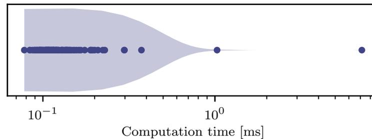
**Figure 9.** Computation times in milliseconds required at runtime to compute a trajectory for each lane center in the evaluation data set. The distribution as a violin plot and the individual samples are displayed.
