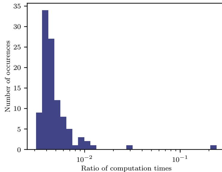
**Figure 10.** Frequency of the ratios of related computation times between the sensitivity-based approach and the re-optimization. For each curve in the evaluation data set, one trajectory was computed using the sensitivity-based approach and one using re-optimization. The thereby observed computation time of the sensitivity-based approach was divided by the time needed for re-optimization.
