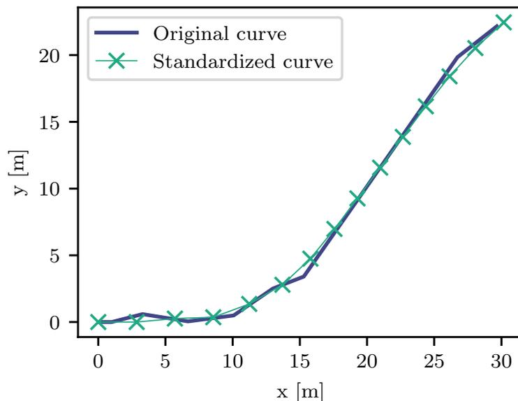
**Figure 3.** Process of standardization: The original curve is one of the cluster centers. The resulting standardized curve complies with the described standardized form.
