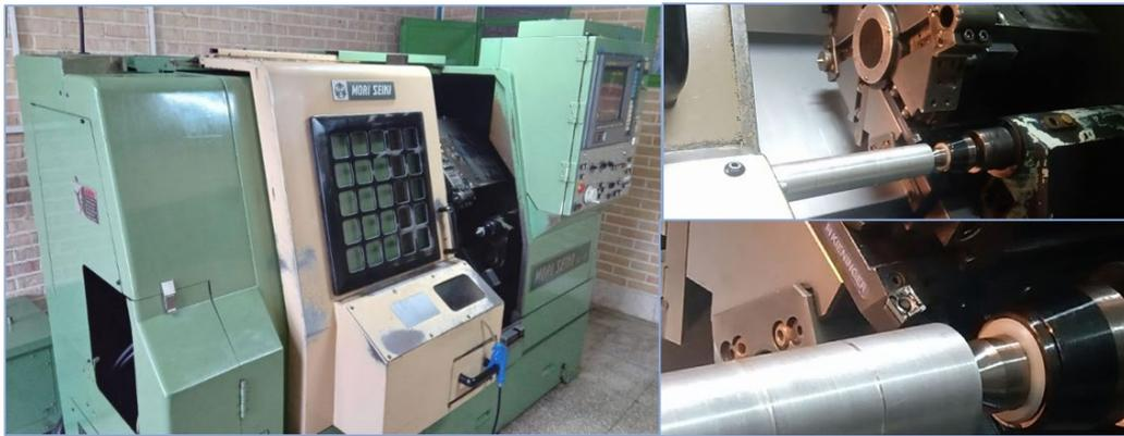
**Figure 8.** The Mori Seiki SL-15 CNC lathe machine and the setup for experimental turning tests.
