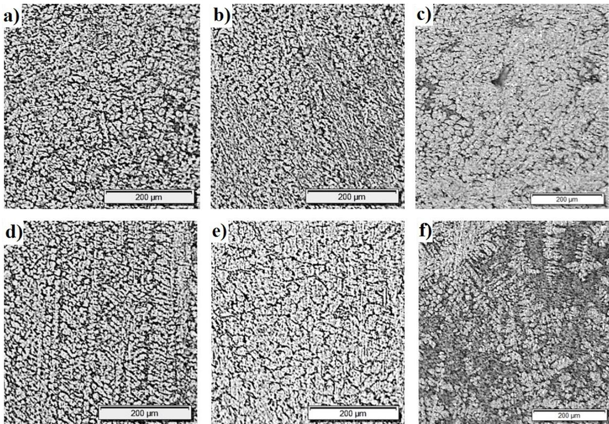
**Figure 2.** Directionally solidified A360 aluminum with solidification velocity of 2 mm/s. (a,d) reference; (b,e)  $B = 0.4$  T; (c,f)  $B = 0.4$  T,  $I = 157$  A.
