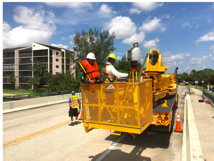
Figure 14. Leica scan station II set up in man basket of snooper truck used for underwater scanning of highway bridge—Little Lake Worth Bridge, Florida.
