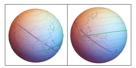
**Figure 1.** The curve of alignment (orange) and the geodesic (blue) from (165 $^{\circ}$  E, 40 $^{\circ}$  S) and (0 $^{\circ}$  E, 45 $^{\circ}$  N) on the WGS 84 reference ellipsoid. The Equator appears in green and the Prime Meridian in orange.
