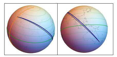
**Figure 3.** The two normal sections (black) and the geodesic (blue) between ( $0^{\circ}$  E,  $45^{\circ}$  N) and ( $165^{\circ}$  E,  $40^{\circ}$  S) on the WGS 84 reference ellipsoid. The Equator appears in green and the Prime Meridian in orange.
