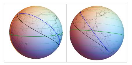
**Figure 5.** The geodesic (blue) and loxodrome (black) from  $(0^{\circ} \text{ E}, 45^{\circ} \text{ N})$  to  $(165^{\circ} \text{ E}, 40^{\circ} \text{ S})$  on the WGS 84 reference ellipsoid. The Equator appears in green and the Prime Meridian in orange.
