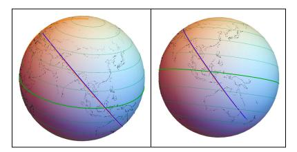
**Figure 4.** Great ellipse (orange) and the geodesic (blue) between ( $0^{\circ}$  E,  $45^{\circ}$  N) and ( $165^{\circ}$  E,  $40^{\circ}$  S) on the WGS 84 reference ellipsoid. The Equator appears in green.
