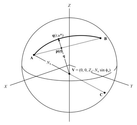
**Figure 2.** The construction of the (shorter limb of the) normal section from **A** to **B**.
