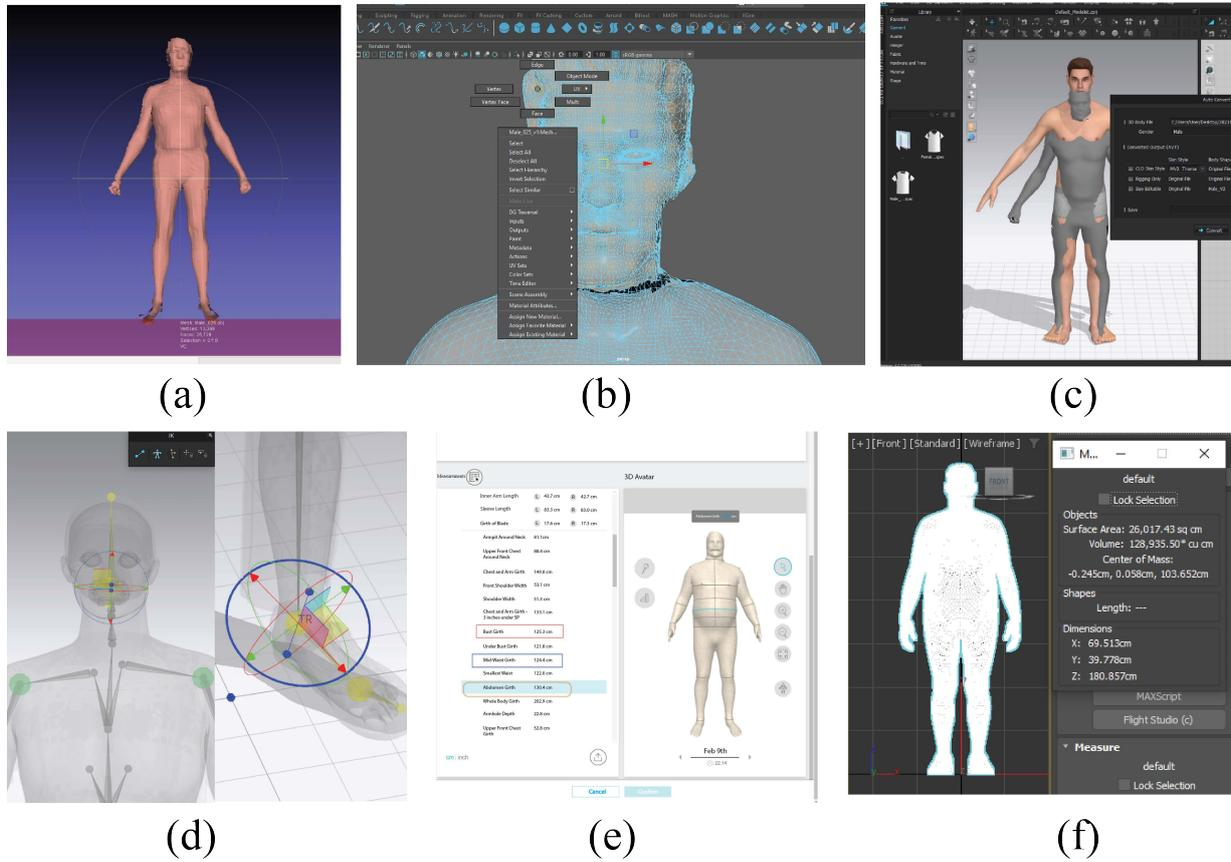
**Figure 2.** 3D avatar development process: (a) Convert body scan files into .obj files in MeshLab; (b) Modify and repair the incomplete surfaces of the scan files in Maya; (c) Convert the scan files into editable .avt files in CLO 3D; (d) Manually adjust joints of avatars in CLO 3D; (e) Extract key body measurements in TG3D Studio; (f) Measure the volume of the avatars in Autodesk 3Ds Max.
