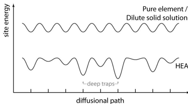
**Figure 4.** Schematic representation of the proposed difference in lattice potential energy profile along an atomic diffusion path in a pure element or dilute solid solution (**top**) and an high-entropy alloy (HEA) lattice (**bottom**). Note it is assumed that the distance between atomic sites is constant. Reproduced from Reference [108]. A similar schematic for the HEA energy profile was given in Reference [105].
