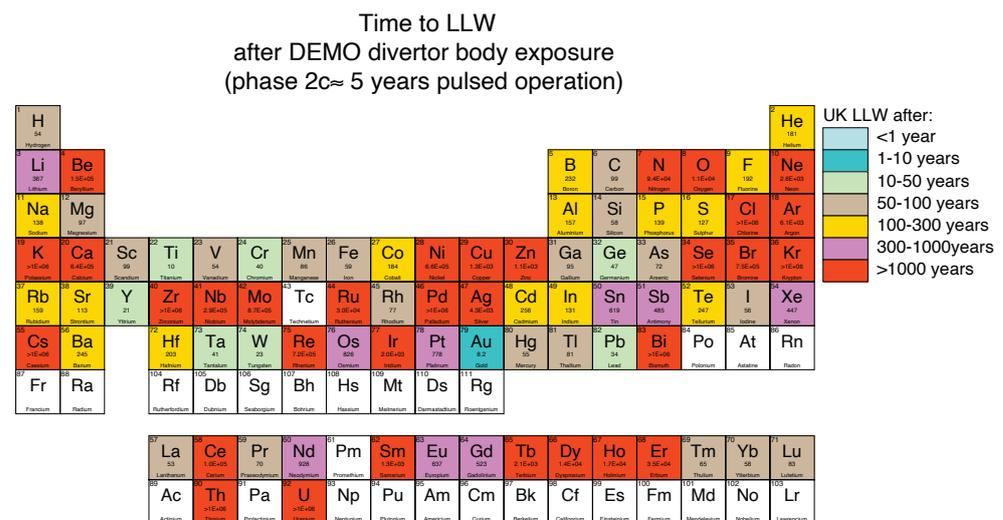
**Figure 2.** Periodic table of the calculated time period that each element would require to decay to UK low level waste limits ( $<4 \text{ MBq kg}^{-1}$  alpha radiation and  $<12 \text{ MBq kg}^{-1}$  combined gamma and beta radiation) following exposure inside a DEMO fusion reactor. The component considered is the divertor over a time period equivalent to 5 years of pulsed operation. Reproduced from Gilbert et al. [15].
