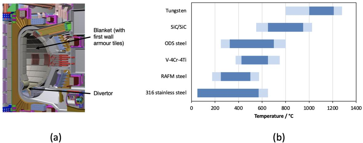
**Figure 1.** (a) Cross section of the ITER tokamak, showing location of first wall, blanket and divertor structures. (b) Operating temperature windows (based on radiation damage and thermal creep considerations) for selected fusion candidate materials. The light shaded bands on either side of the dark bands represent the uncertainties in the temperature limits. This figure is a modified version of that first presented in Reference [8].
