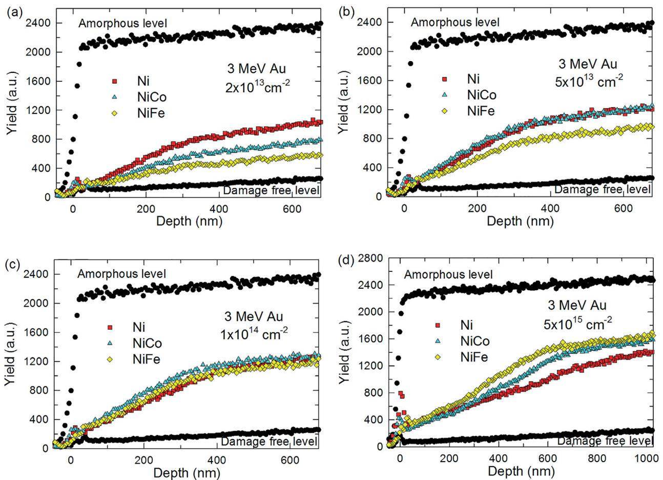
**Figure 3.** Rutherford backscattering channeling spectra of Ni, NiCo and NiFe, irradiated with 3 MeV Au ions to the fluences ranging from  $2 \times 10^{13}$  (a),  $5 \times 10^{13}$  (b),  $1 \times 10^{14}$  (c) to  $5 \times 10^{15}$  (d) ions  $\text{cm}^{-2}$  Reproduced from Reference [80].
