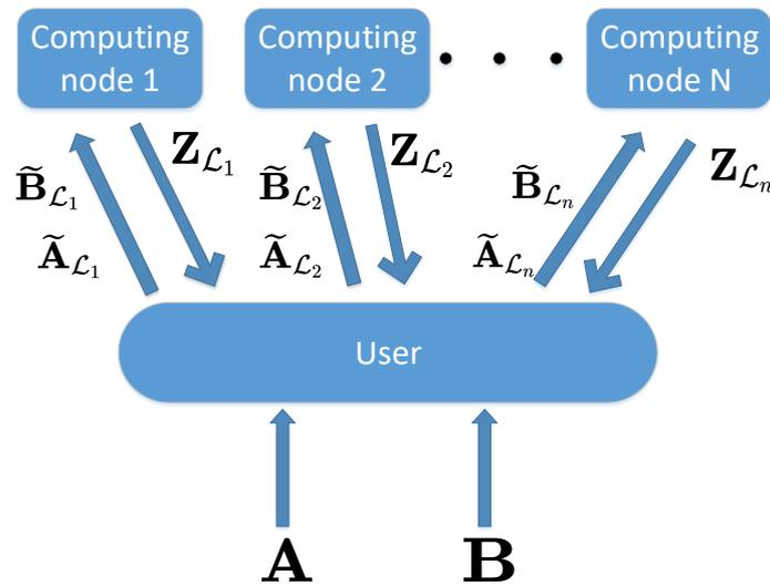
**Figure 1.** Two-sided secure distributed matrix multiplication.
