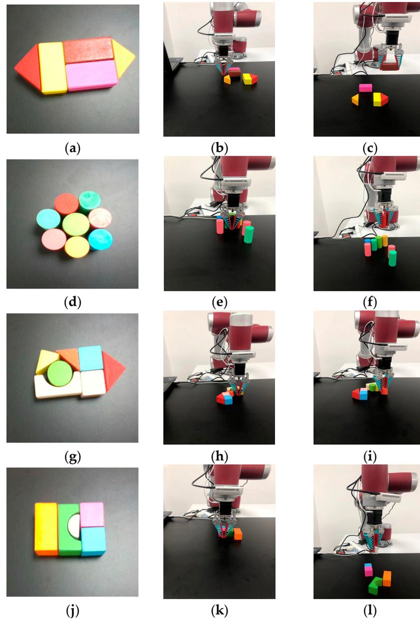
**Figure 13.** The grasping experiments of multiple unknown objects in real world.
