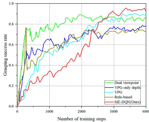
**Figure 11.** The comparison of training for novel unknown objects with benchmarks in simulation.
