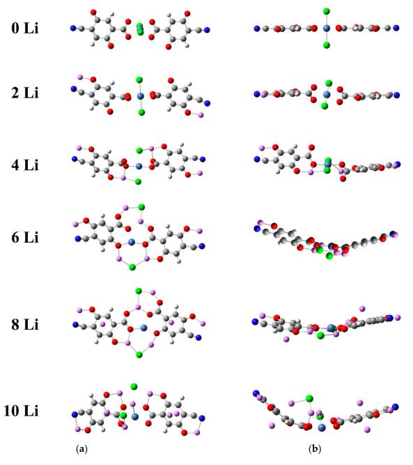
**Figure 4.** Stages of lithiation of Ni(IV)(L1)<sub>2</sub>—(**a**) top and (**b**) side view of the optimized geometries. Color code: C—gray, H—white, O—red, N—deep blue, Ni—light blue, Cl—green, Li—pink.
