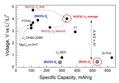
**Figure 15.** Voltage-capacity plot of organic-based electrode materials reported in the literature (PTPAn [51], Li<sub>4</sub>-p-DHBD.2DMF [47], Mg(Li<sub>2</sub>)-p-DHT [52], Li<sub>2</sub>-BDC [53] and ZnTPA [54]—black labels and circles), and in this study (colored labels, full circles for the high potential and patterned circles for the low potential); the most prospective structures designed in this study (in red) for the construction of an all-organic rechargeable Li-ion battery.
