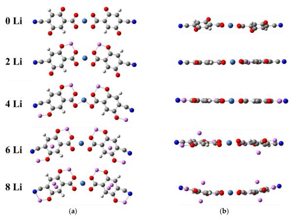
**Figure 2.** Stages of lithiation of Ni(II)(L1)<sub>2</sub>—top (**a**) and side (**b**) view of the optimized geometries. Color code: C—gray, H—white, O—red, N—deep blue, Ni—light blue, Li—pink.
