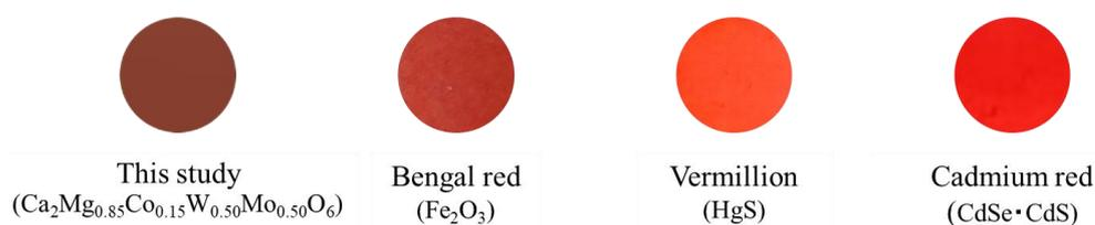
**Figure 13.** Photographs of  $\text{Ca}_2\text{Mg}_{0.85}\text{Co}_{0.15}\text{W}_{0.50}\text{Mo}_{0.50}\text{O}_6$ , Bengal red, vermilion, and cadmium red pellets made from powder samples.
