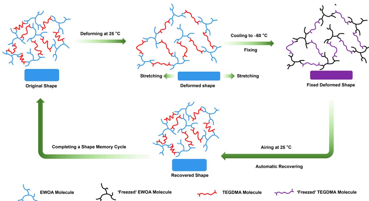
**Figure 7.** Schematic illustration of the structural transformation in EWOA-TEGDMA resin during a shape memory cycle.
