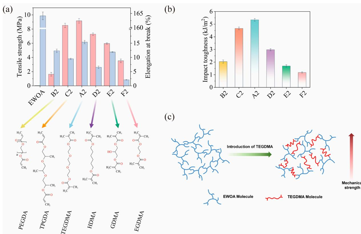
**Figure 3.** (a,b) Tensile properties (a) and impact toughness (b) of pure EWOA and WCO-based 4D-printable resins composed of EWOA and different diacrylate molecules; (c) Schematic illustration of the structural differences between the curing products of EWOA-TEGDMA resin and pure EWOA.
