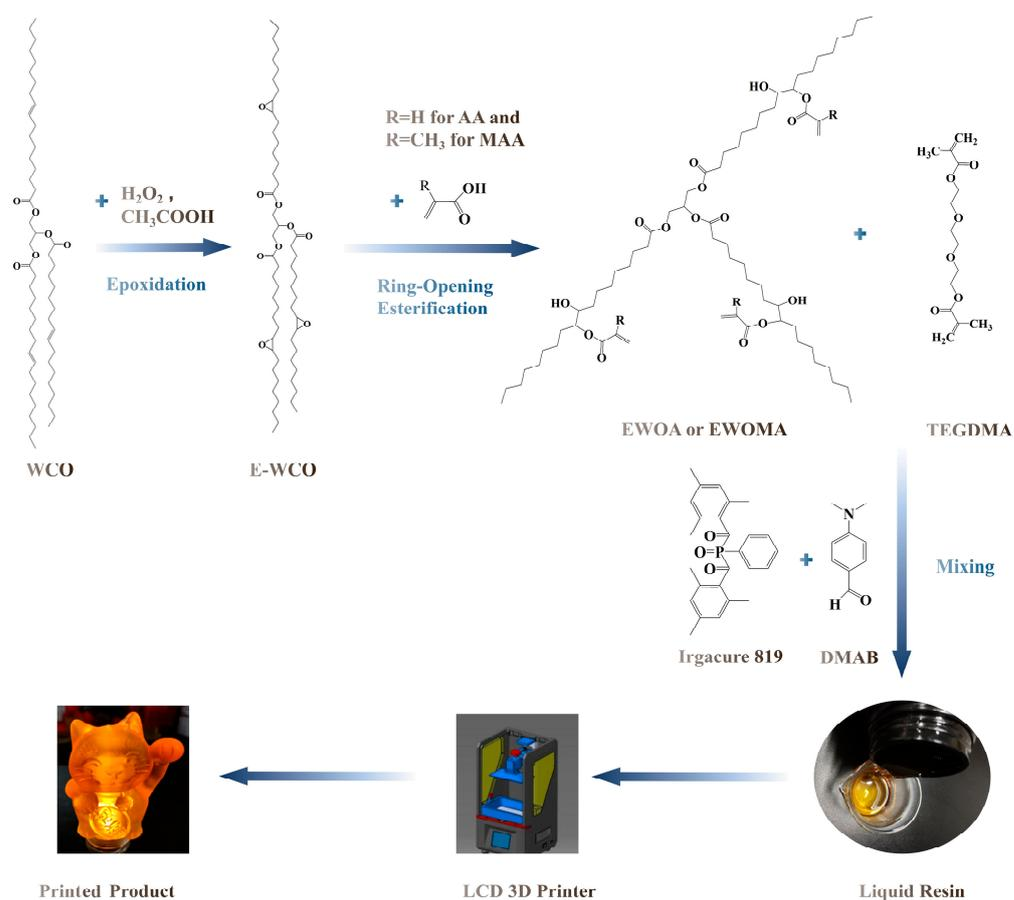
**Figure 1.** Schematic illustration of the preparation and 4D printing process of the WCO-based photocurable resin.
