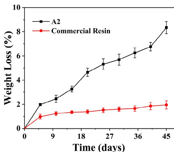
**Figure 8.** Biodegradation rates of EWOA-TEGDMA resin (A2 sample) and commercial 3D printing resin measured by the weight loss.
