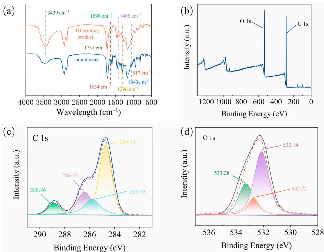
**Figure 2.** (a) IR spectra of 4D-printed product and liquid resin of A2 sample; (b–d) The full XPS (b), C1s (c), and O1s (d) high-resolution XPS spectra of 4D-printed product of A2 resin.
