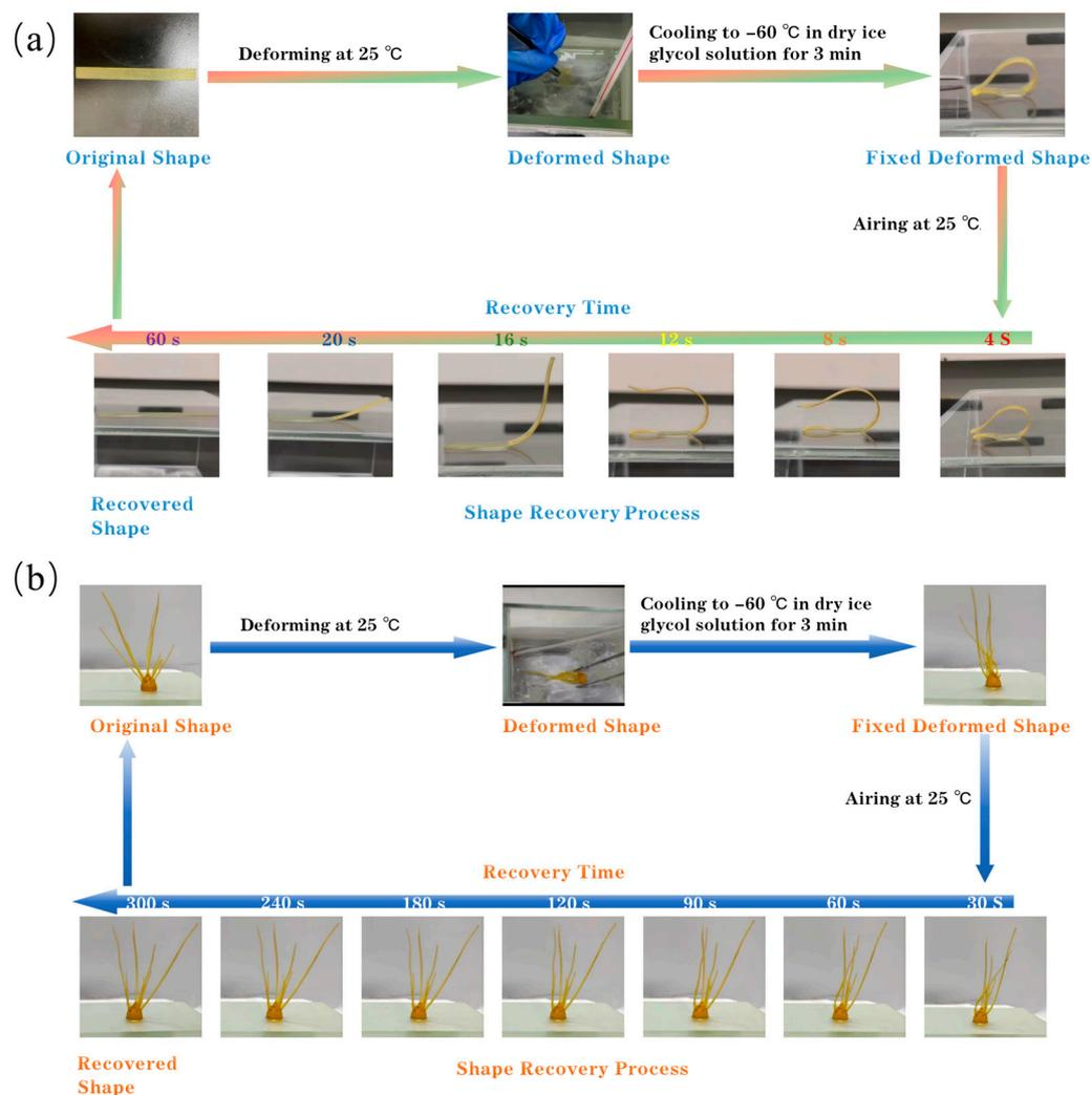
**Figure 5.** Shape memory cycle of a 4D-printed rectangular thin film (a) and radish roots (b) of A2 resin.
