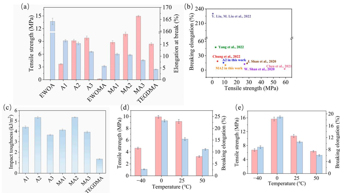
**Figure 4.** (a,c) The tensile properties (a) and impact toughness (c) of EWOA/EWOMA-TEGDMA resins with different dosages of TEGDMA at room temperature; (b) The comparison of mechanical properties between the resulting WCO-based resin (A2 and MA2 sample) and other petroleum-based photocurable resins for 4D printing; (d,e) The tensile properties of the A2 (d) and MA2 (e) resin at different temperatures.
