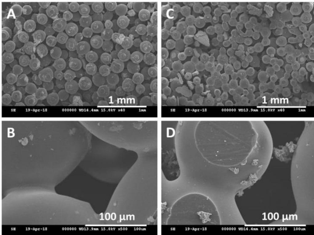
**Figure S4.** The SEM images of low and high magnification of PLGA/nHAP microsphere scaffold (A and B) and PLGA/nWLKT microsphere scaffold (C and D).
