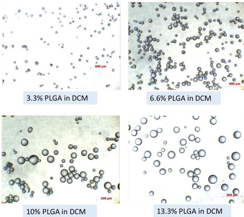
**Figure S2.** The optical microscopic images of PLGA microspheres obtained at different PLGA concentrations for the optimization of PLGA concentration.
