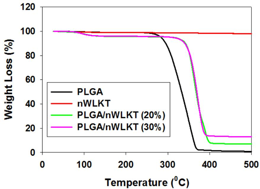
**Figure S3.** The TGA results for the assay conducted for microsphere scaffold containing two different concentrations of nWLKT for the optimization of nWLKT loading.
