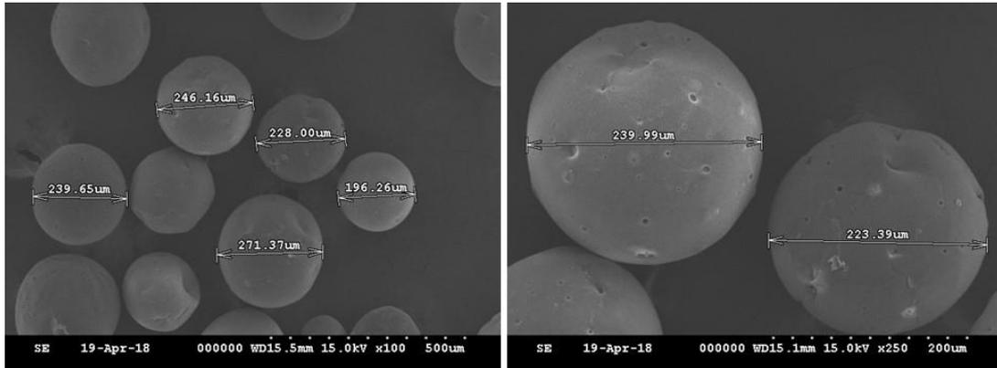
**Figure S1.** The SEM images of PLGA microspheres at different magnifications.
