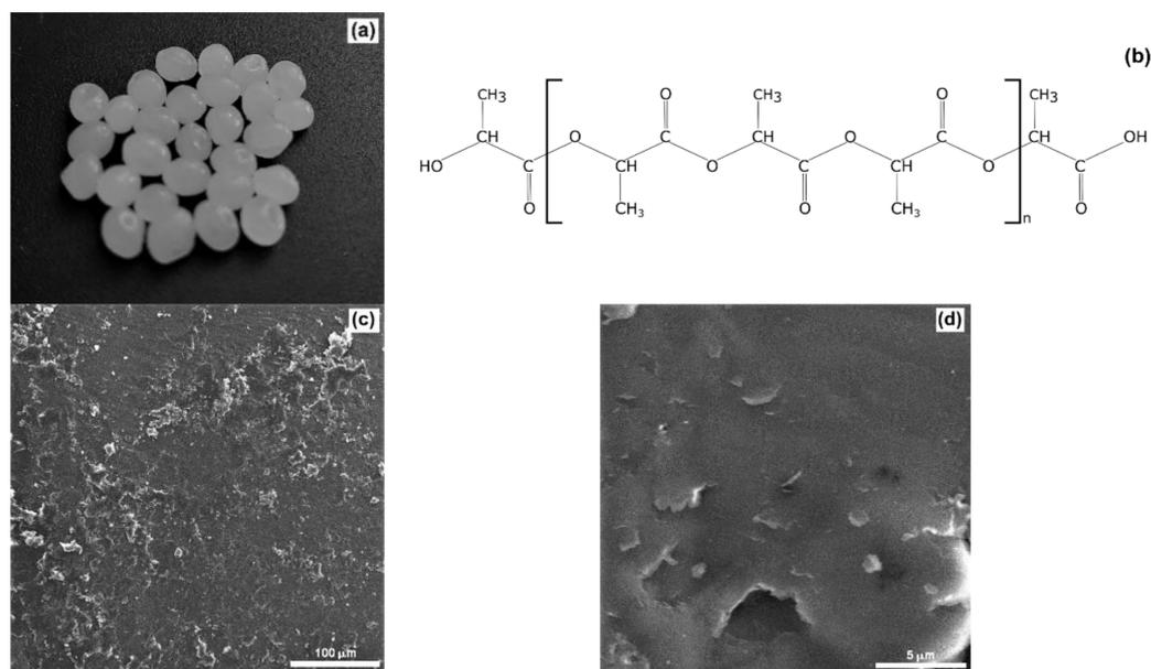
**Figure 1.** (a) Photograph of PLA granules, (b) structural formula of PLA and (c,d) SEM images of PLA at different magnifications.
