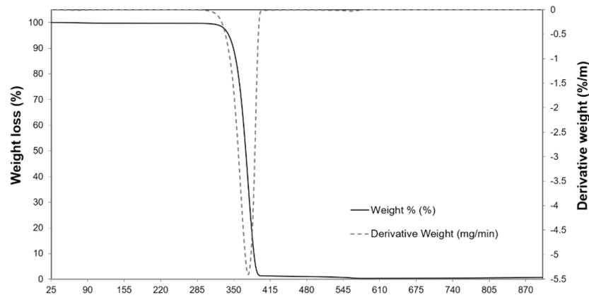
**Figure 2.** Thermogravimetric analysis (TGA)/differential thermogravimetric (DTG) analysis of PLA.
