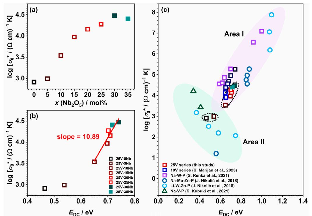
**Figure 9.** The dependence of the pre-exponential factor ( $\sigma_0^*$ ) as a function of (a) composition and (b) activation energy ( $E_{DC}$ ); and (c) a comparison of the glasses and glass–ceramics from this study with those from 10V series [27] and systems Na-W-P [22], Na-Mo-Zn-P [25], Li-W-Zn-P [25] and Na-V-P [23] from the literature. The line in (b) is obtained through linear regression. The dotted circles in Figure 9c highlight the samples from this study.
