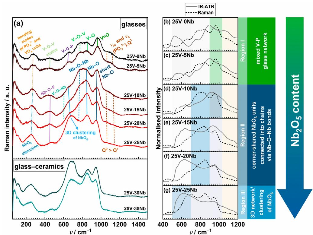
**Figure 4.** (a) Raman spectra of glasses and glass–ceramics from the 25V series and (b–g) comparison of IR-ATR and Raman spectra for individual glass samples. Shading in (b–g) corresponds to the band assignment in (a). The orange shade denotes the vibration of phosphate units, the green shade represents vanadate units, and the blue shade indicates niobate units. The most intense colored regions correspond to the dominant signals.
