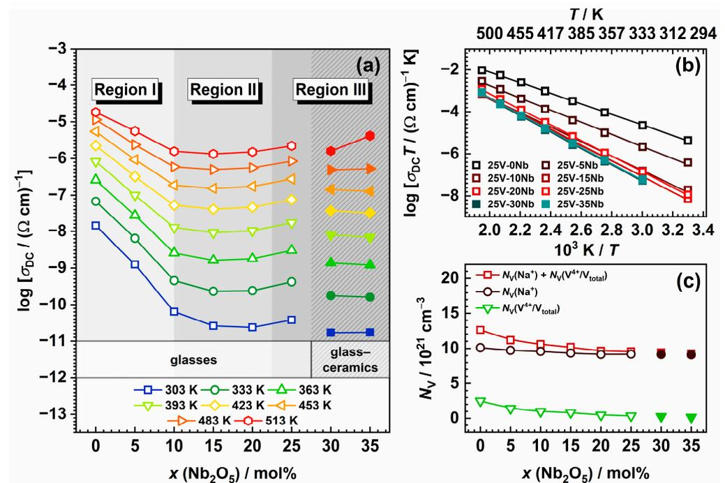
**Figure 6.** (a) Compositional and temperature dependence of DC conductivity,  $\sigma_{DC}$ ; (b) Arrhenius plot of DC conductivity; and (c) compositional dependence of number density,  $N_V$ , of  $\text{Na}^+$  ions,  $\text{V}^{4+}$  ions, and the total number density of charge carriers. Empty symbols represent glasses, whereas full symbols denote glass-ceramics. The lines connecting data points in (a,c) are a guide for the eye, while the lines in (b) are obtained through linear regression.
