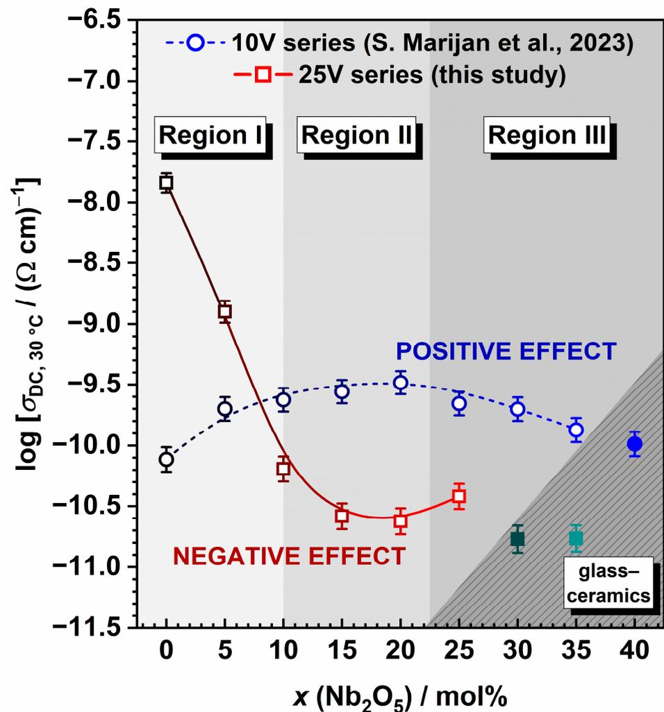
**Figure 8.** Comparison of compositional dependence of DC conductivity,  $\sigma_{DC}$ , at 303 K for two glass and glass-ceramics series,  $35Na_2O-10V_2O_5-(55-x)P_2O_5-xNb_2O_5$  [27] and  $35Na_2O-25V_2O_5-(40-x)P_2O_5-xNb_2O_5$ . The lines connecting data points are a guide for the eye.
