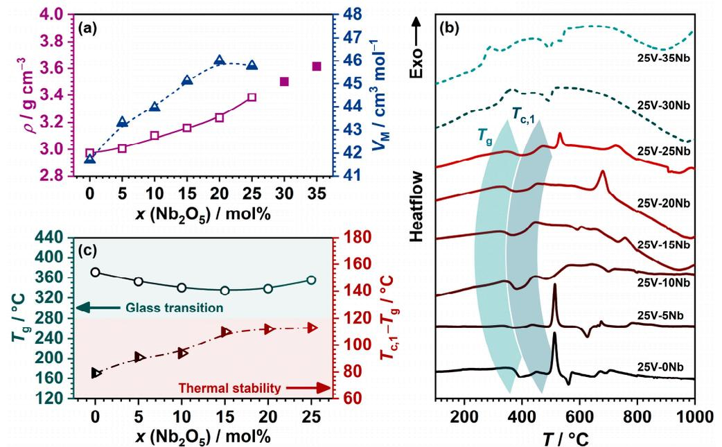
**Figure 1.** (a) Dependence of density,  $\rho$ , and molar volume,  $V_M$ , on Nb<sub>2</sub>O<sub>5</sub> content; (b) DTA curves; and (c) dependence of glass transition temperature,  $T_g$ , and the parameter ( $T_c - T_g$ ) on Nb<sub>2</sub>O<sub>5</sub> content. The lines connecting data points in (a,c) are a guide for the eye.
