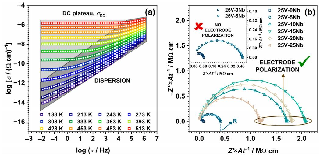
**Figure 5.** (a) Conductivity spectra at different temperatures for 25V-20Nb glass and (b) the complex impedance spectra for all glass samples at 483 K. Empty symbols represent the experimental data, while the lines depict the fit obtained through EEC modelling.
