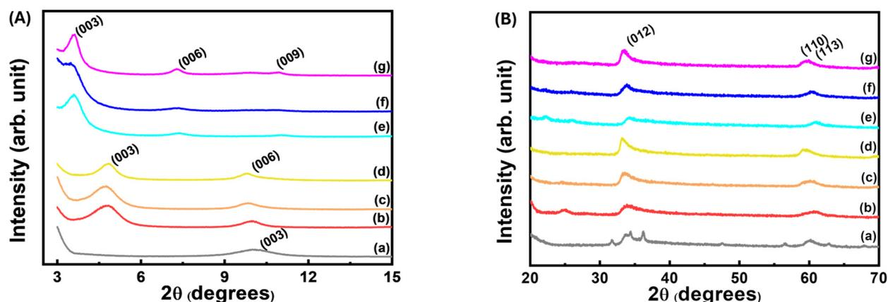
**Figure 1.** X-ray diffraction patterns in the high-angle region for (a) ZnAl-NO $_3$ -LDH, (b) CL1, (c) CL2, (d) CL3, (e) CLC1, (f) CLC2, and (g) CLC3. (A) low  $2\theta$  region and (B) high  $2\theta$  region.
