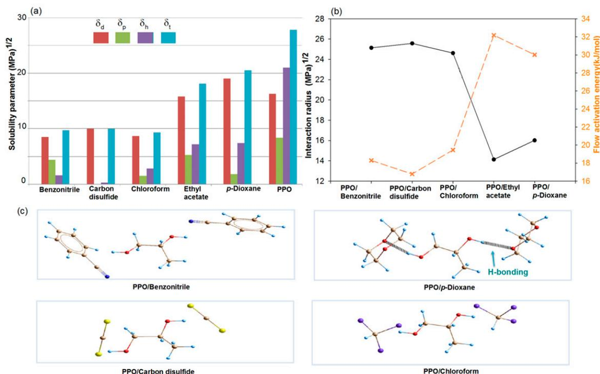
**Figure 2.** Solubility parameter components for the used solvents and those calculated for PPO (a), variation of the interaction radius (continuous line) and flow activation energy (dash line) (b) for all studied PPO solutions, and (c) interaction representation of the PPO structural unit in the presence of two solvent molecules (dashed line shows the hydrogen bonding between the PPO and the solvent).
