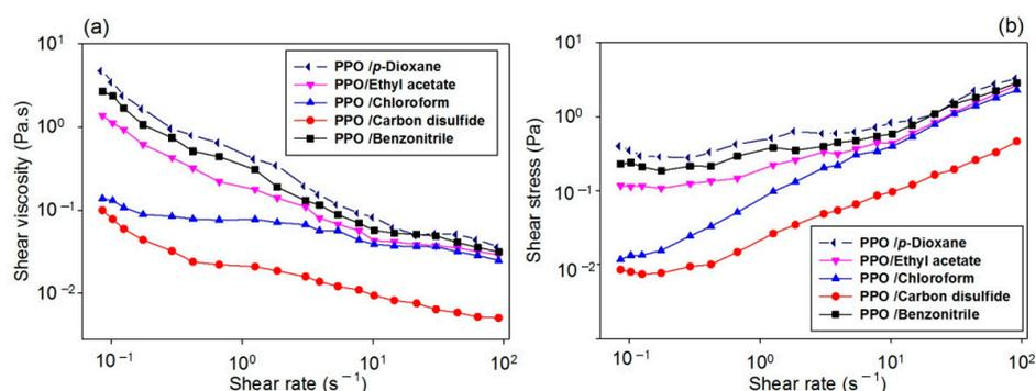
**Figure 1.** Dependence of (a) shear viscosity and (b) shear stress on shear rate for PPO solutions in several solvents.
