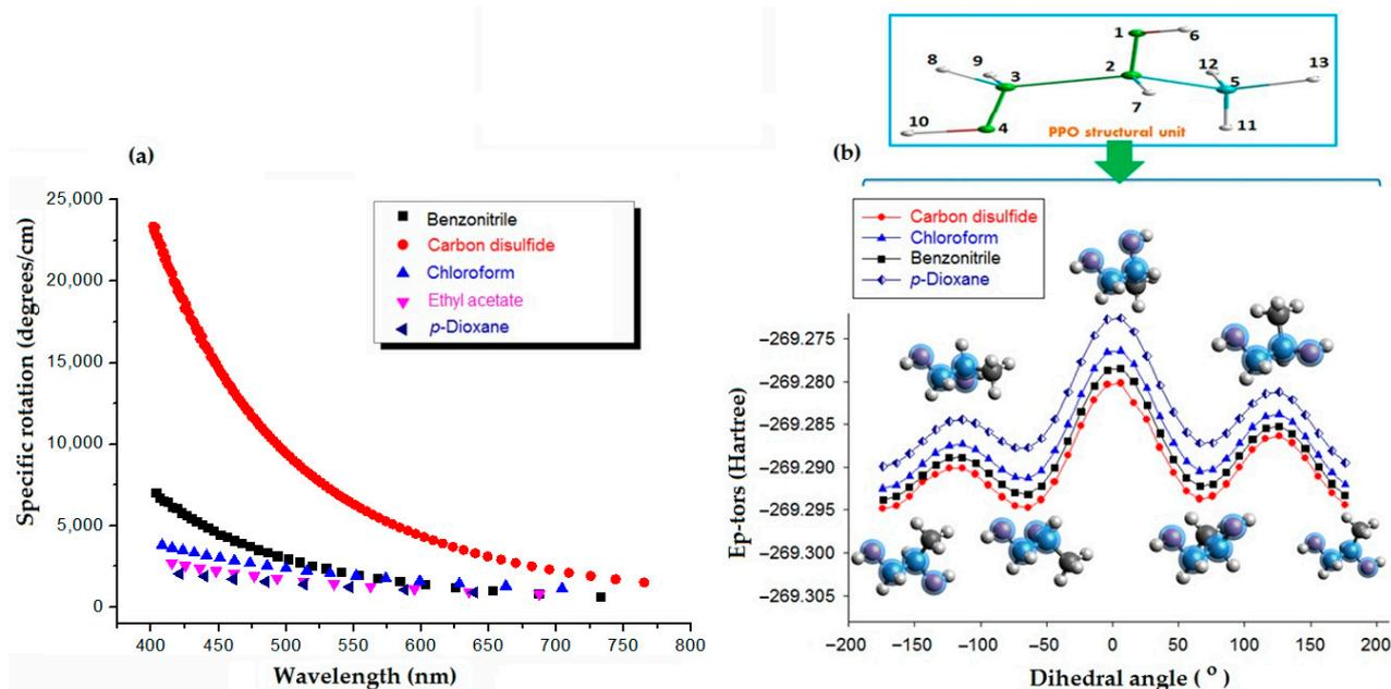
**Figure 7.** The specific rotation obtained for PPO in several solvents (a) and the representation of the optimized configuration of the PPO structural unit with atom order and the torsional potential energy profile versus the O1-C2-C3-O4 dihedral angle from PPO structural unit in the presence of the studied solvents (the numbers from the upper inset index the atoms of the PPO structural unit) (b).
