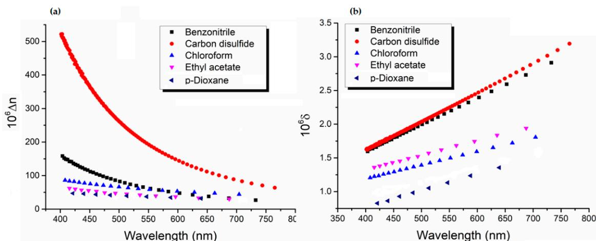
**Figure 6.** Circular birefringence dispersion (a) and birefringence dispersion parameters (b) obtained for PPO in several solvents.
