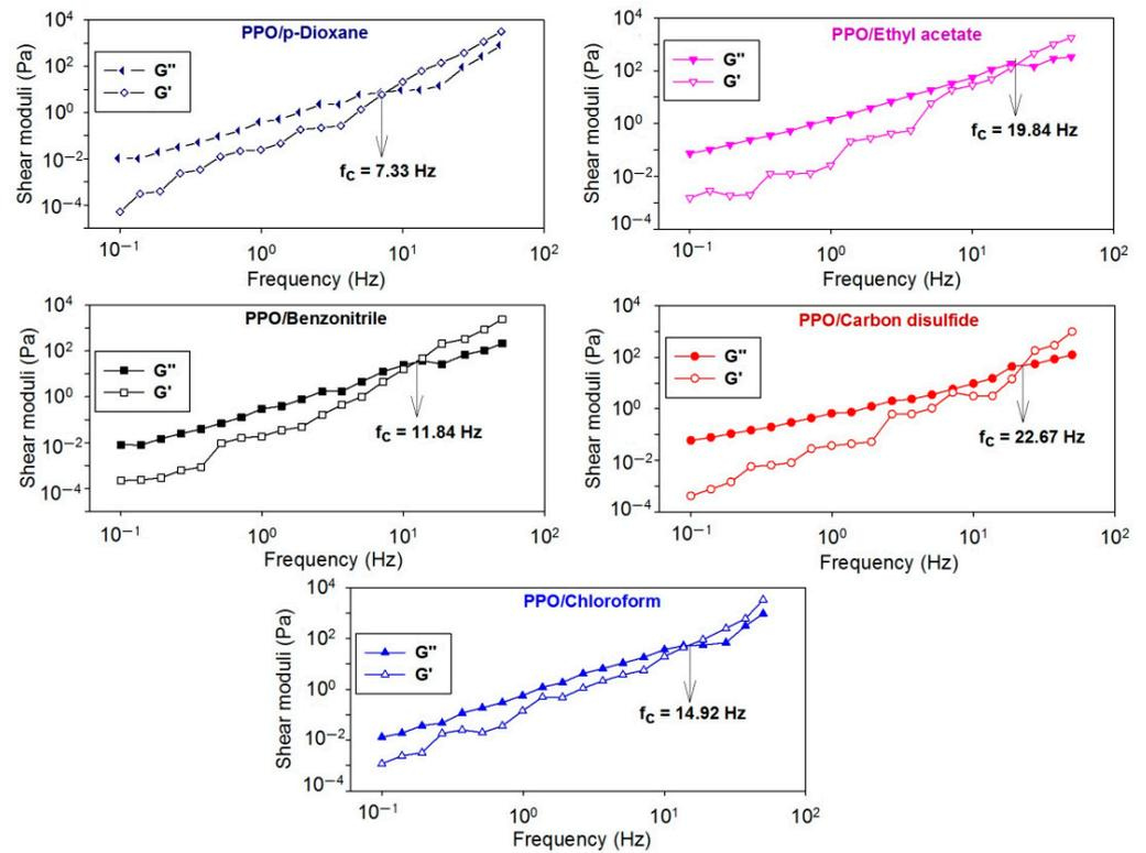
**Figure 3.** Shear oscillatory tests of the PPO solutions in several solvents.
