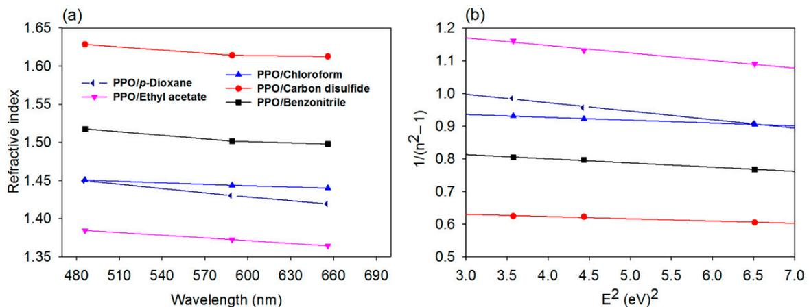
**Figure 4.** Refractive index dispersion (a) and  $1/(n^2 - 1)$  against the square photon energy ( $E^2$ ) (b) for the PPO solutions in several solvents.
