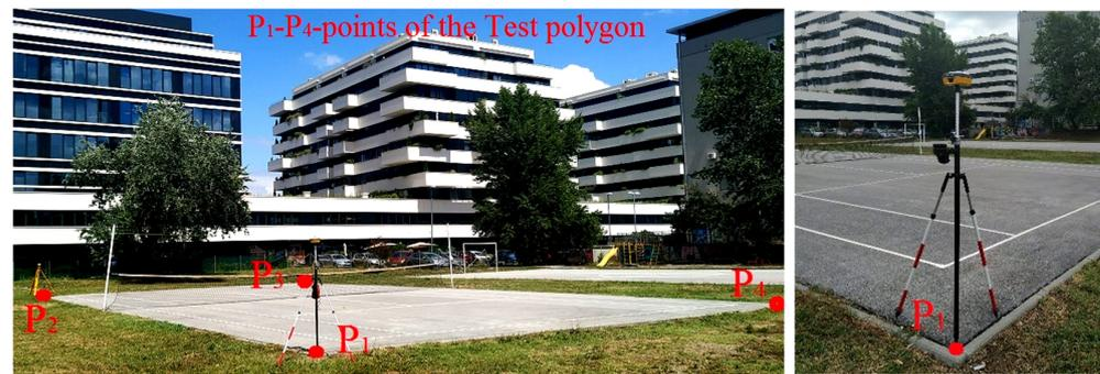
**Figure 5.** Measurements in the Test polygon—GNSS RTK mode (point  $P_1$  of the Test polygon).
