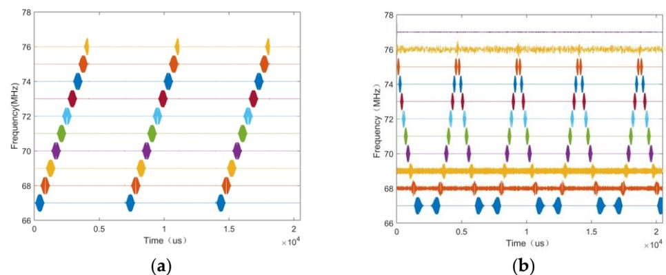
**Figure 4.** Wave-frequency diagrams of different signals ((a): LFM; (b): EQFM + BPSK + DQPSK + 8PSK).
