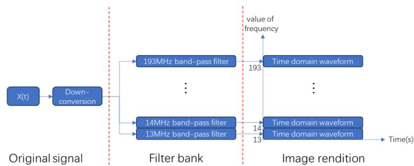
**Figure 3.** Flowchart for generating wave-frequency diagrams.
