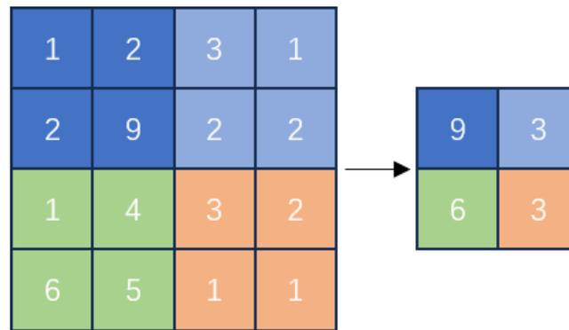
**Figure 15.** Schematic of maximum pooling.
