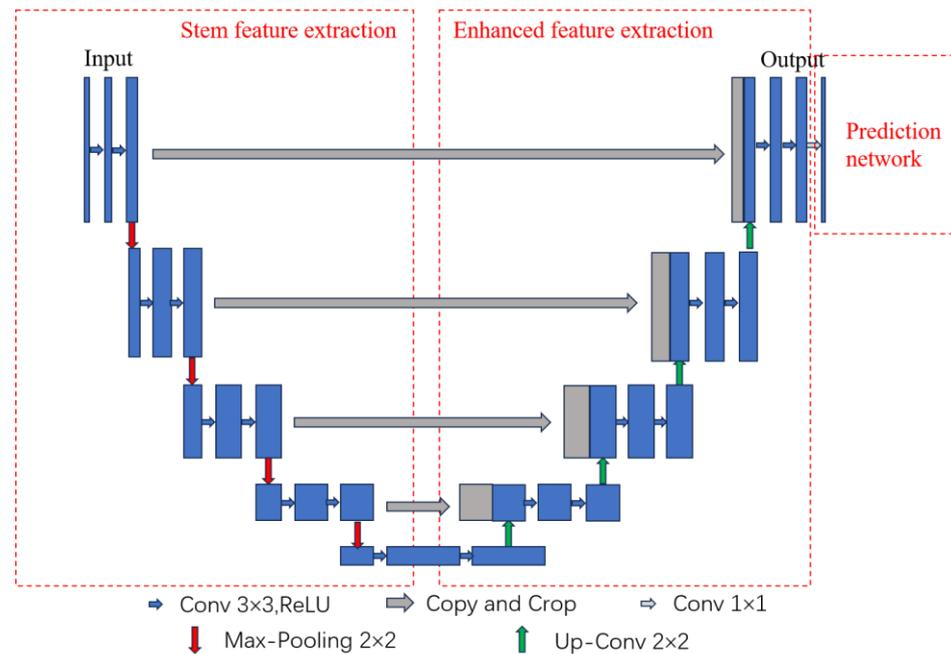
**Figure 13.** Structure of the U-Net network.
