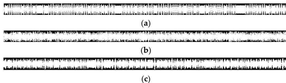
Figure 11. Wave-frequency diagram of MPSK signal ((a): BPSK; (b): QPSK; (c): 8PSK).
