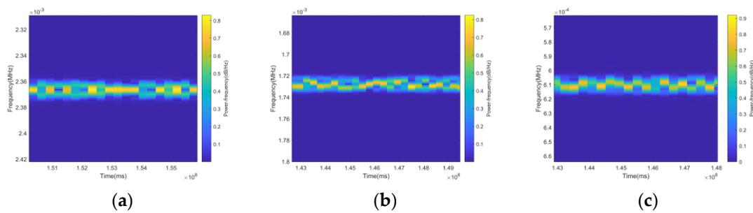
Figure 10. Time-frequency diagram of MPSK signal ((a): BPSK; (b): QDPSK; (c): 8PSK).
