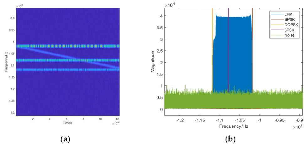
**Figure 6.** Time-frequency diagram and corresponding spectrum of BPSK + DQPSK + 8PSK + LFM model ((a). time-frequency distribution, (b). spectrum waveform).
