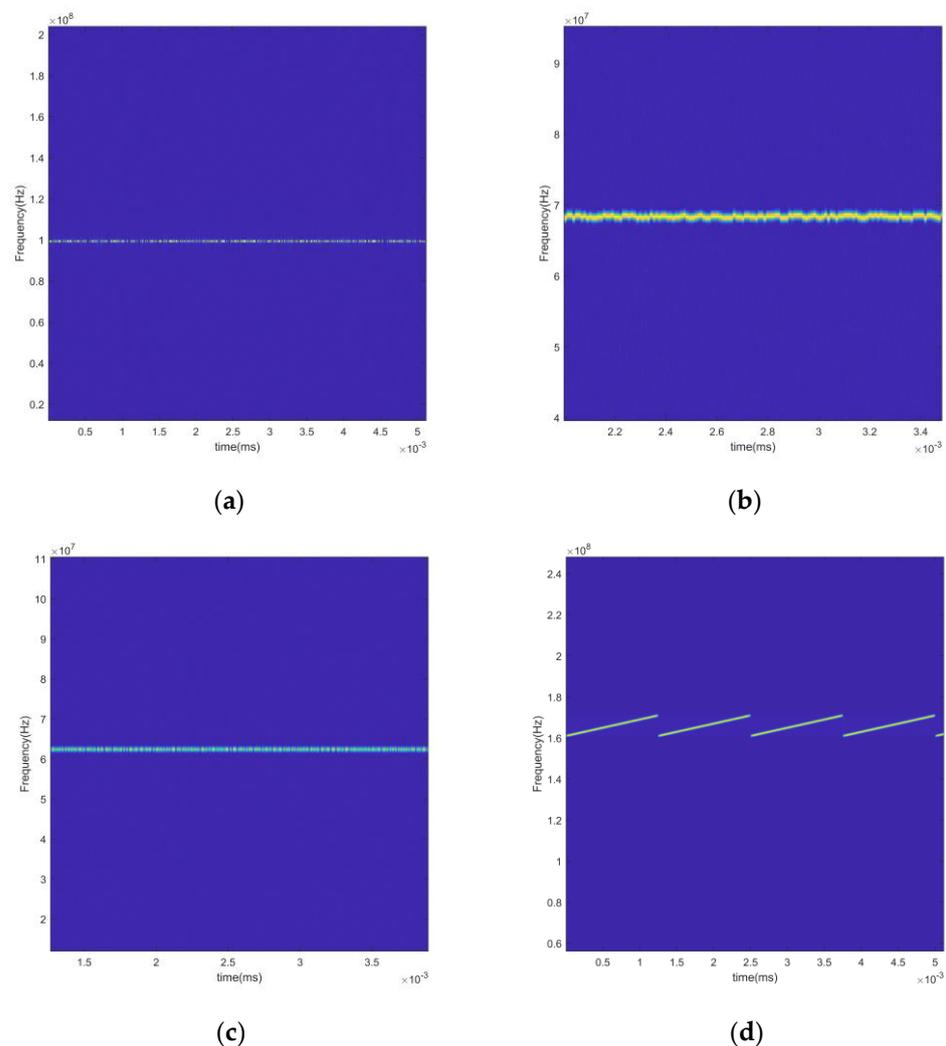
**Figure 2.** Example of time-frequency diagrams for different signals ((a): 2ASK; (b): 4FSK; (c): 8PSK; (d): EQFM).
