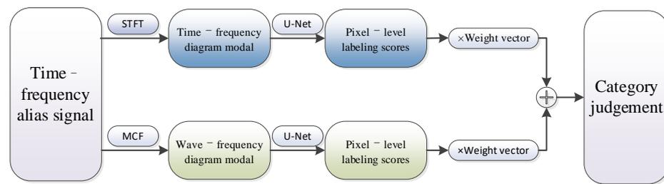
Figure 9. Basic flowchart of TRMM method processing.
