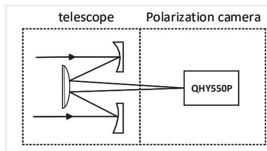
**Figure 3.** Optical system configuration of the experiment mounting.
