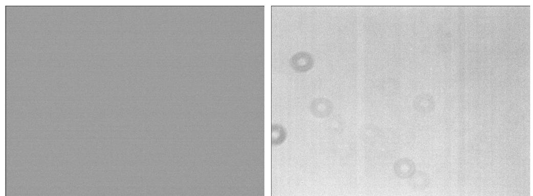
**Figure 5.** Auxiliary bias and flat images. (a) Combined bias: median image of 10 bias images. (b) Combined flat: median image of 10 flat-field images.
