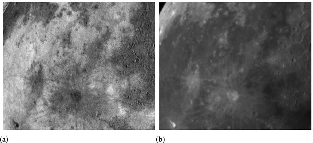
**Figure 7.** DOP image and light intensity image are calculated by the Stokes formula. (a) DOP image. (b) Light intensity image.
