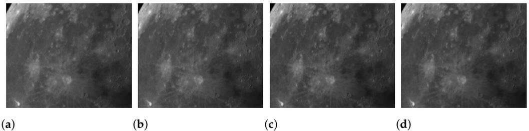
**Figure 2.** Four-directional polarization information captured in one shot: (a) 0-degree polarization direction sub-image; (b) 45-degree polarization direction sub-image; (c) 90-degree polarization direction sub-image; (d) 135-degree polarization direction sub-image.
