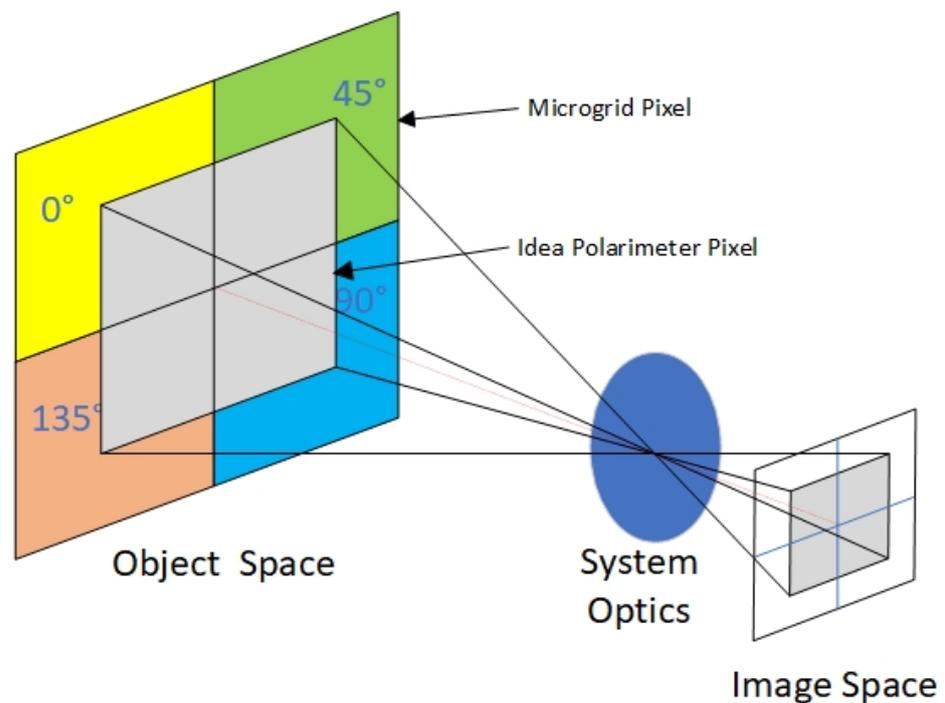
**Figure 6.** Schematic diagram of the instantaneous field of view error in the defocusing plane [27]. The ideal polarimeter pixel is capable of measuring the same area in space over the same interval in time for each polarizer orientation. IFOV error arises due to differences in the captured spatial areas or timing intervals captured by the ideal polarimeter pixel and the microgrid pixels.
