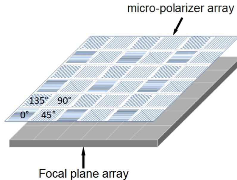
**Figure 1.** Schematic structure of a DoFP sensor.
