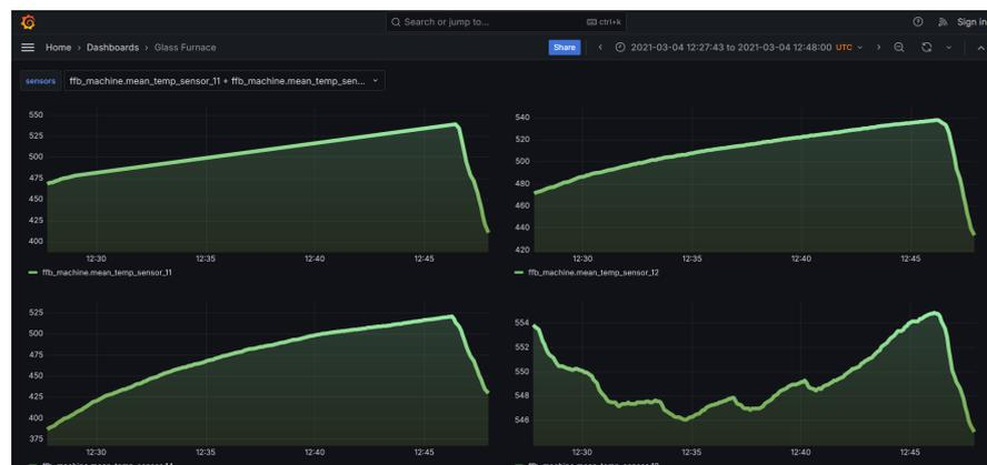
Figure 9. Grafana dashboard for thermal couple temperature visualization.
