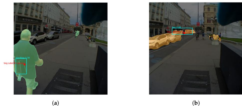
**Figure 3.** As an example, these images show the different semantic recognition levels of the two models and how beneficial this feature can be for some applications. (a) Mask2Former recognizes the person, but YOLO also recognizes the handbag the person is carrying. (b) Mask2Former recognizes a car queue, but YOLO correctly recognizes the bus in the queue.
