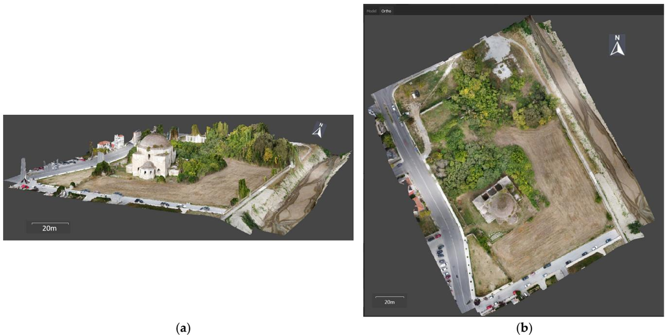
Figure 19. Products of the UAV image processing for the historical complex: (a) 3D photogrammetric model; (b) orthophotomosaic.
