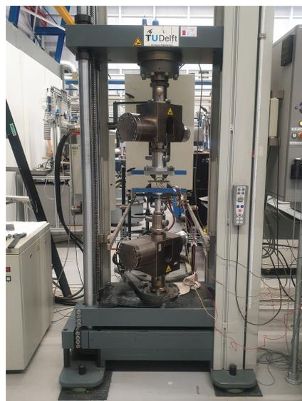
Figure 6. The Zwick 250 kN test bench.
