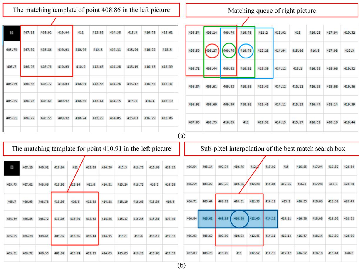
**Figure 6.** Schematic of the sub-pixel stereo matching (a) Select any point on the left phase diagram to create a  $3 \times 3$  matching template, and search for a matching queue on the right phase diagram. (b) Select the two pixels before and after the best matching search box to perform cubic spline interpolation.
