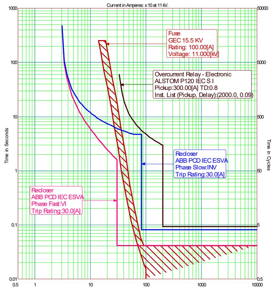
**Figure 6.** Coordination curves using IDMT characteristics between the OCR, recloser, and fuse.
