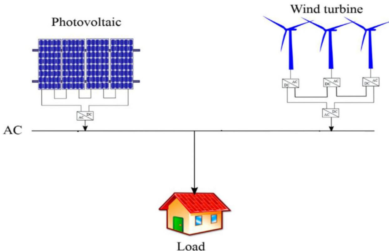
**Figure 2.** A schematic diagram of a grid-connected GDG.
