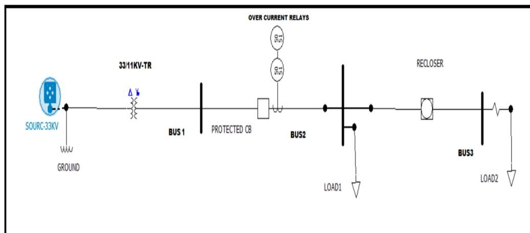
**Figure 5.** Medium voltage 11 kV model in RDNs.
