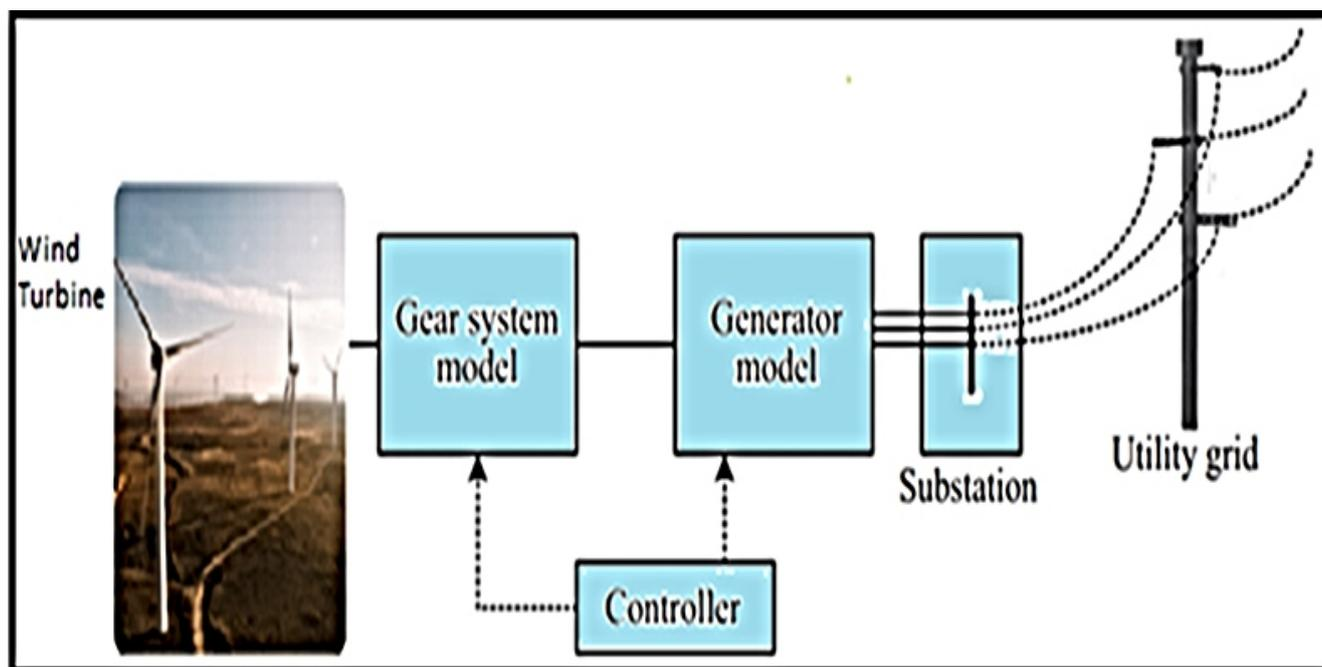
Figure 11. A simplified WT system block diagram.
