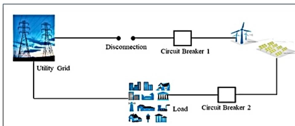
**Figure 3.** Loss of main (LOM).
