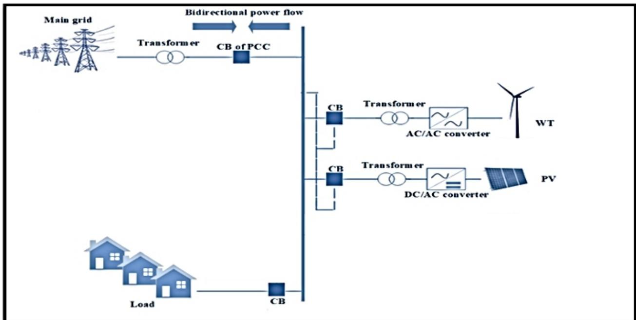
Figure 9. Structure of a  $\mu$ G.
