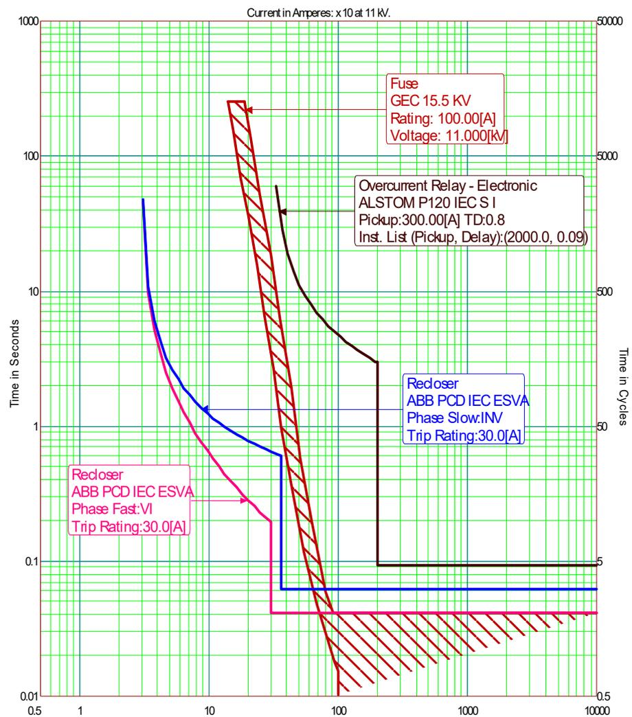
Figure 8. Coordination curves using IDMT characteristics between the OCR, recloser, and fuse with connected PV solar.
