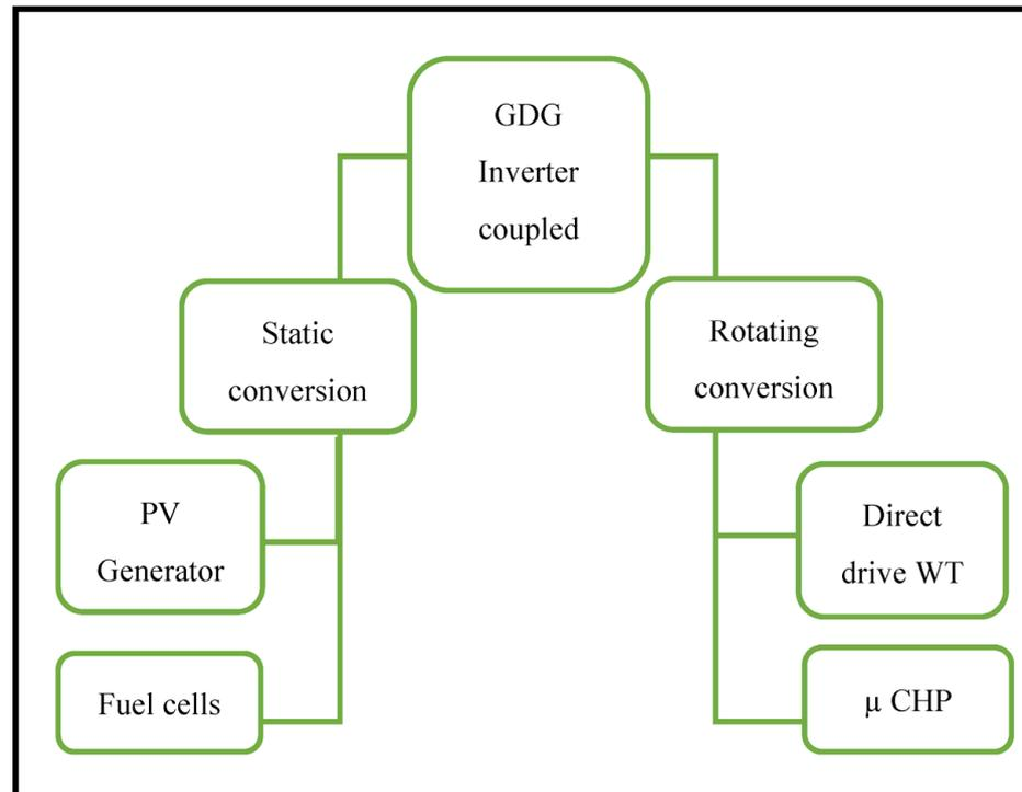
**Figure 1.** Classification of GDG inverter coupled.
