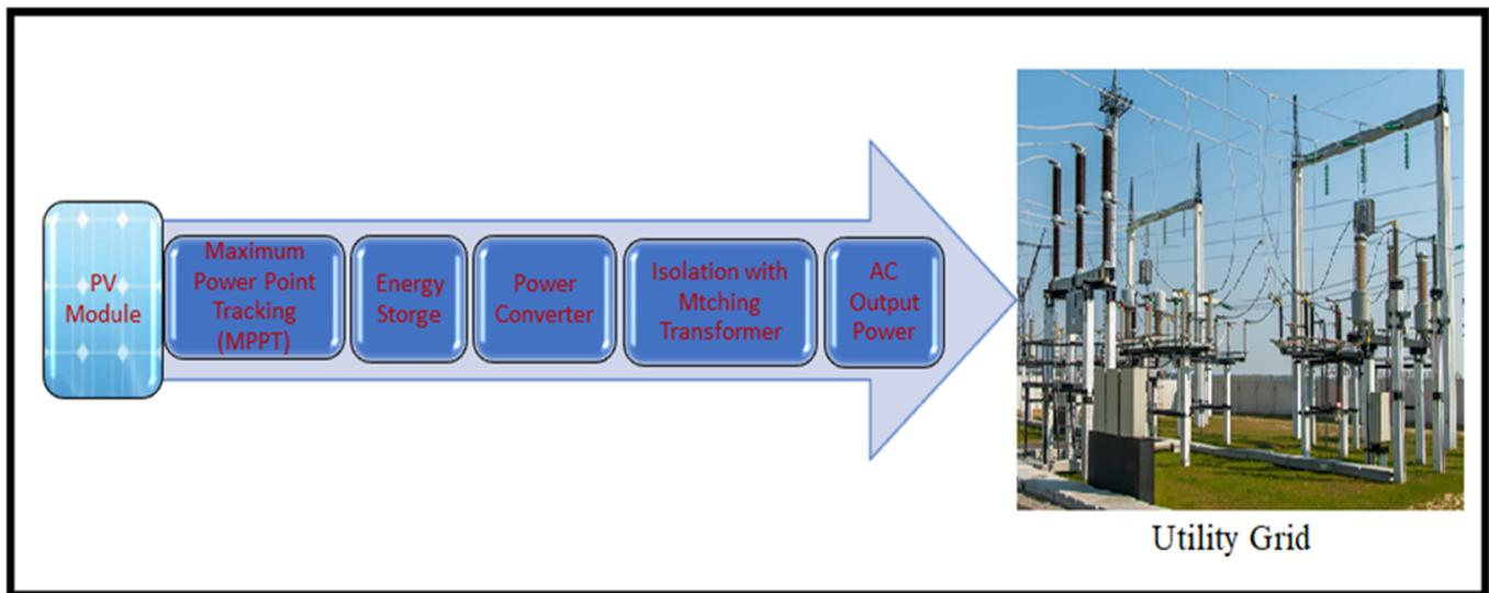
**Figure 10.** A grid-connected photovoltaic system hardware structure.
