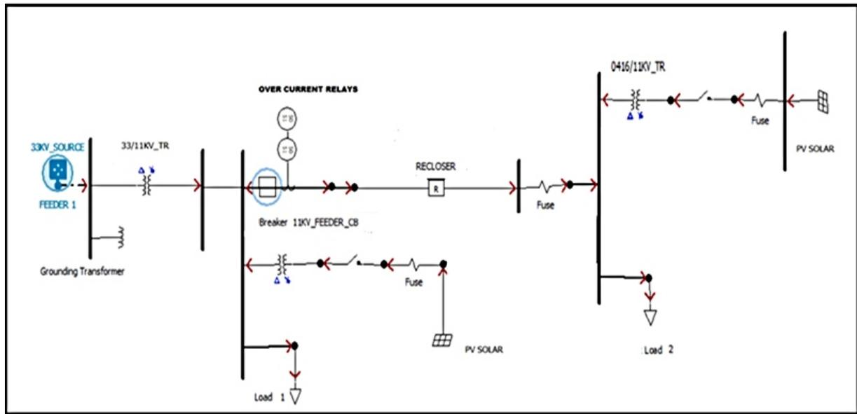
Figure 7. Medium voltage 11 kV model in RDNs with PV solar.
