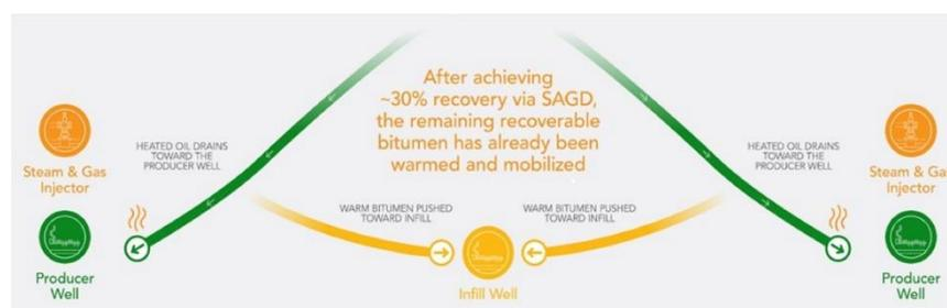
**Figure 2.** Schematic diagram of EMVAPEX [23].
