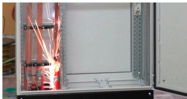
**Figure 6.** Short-circuit test results with two jumpers mounted—30 kA RMS: moment of recorded arcing and displacement of the busbar.
