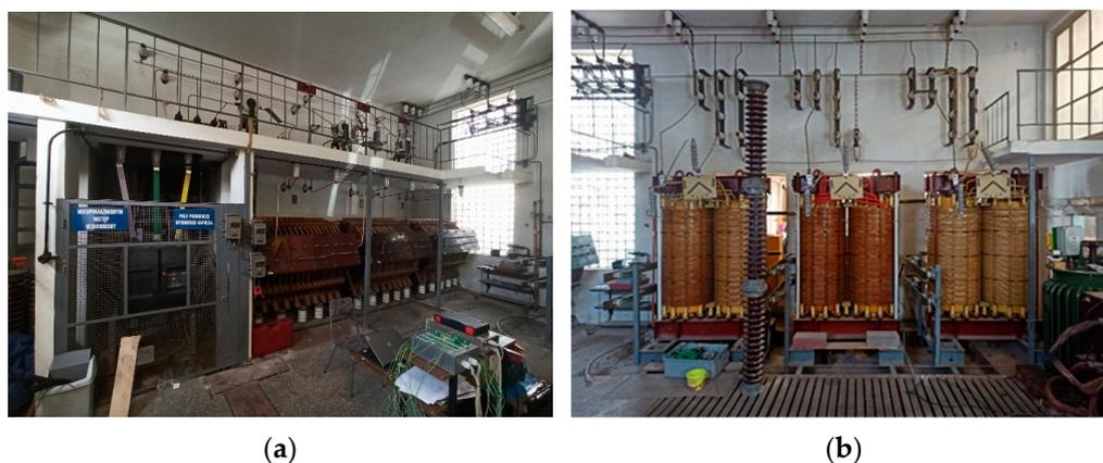
**Figure 3.** Short-circuit system in the Distribution Equipment Laboratory of the Institute of Power Engineering where short-circuit tests of the LV switchgear were performed: (a) short-circuit reactors; (b) short-circuit transformers.
