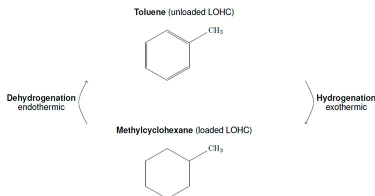
**Figure 5.** Storage cycle of the LOHC system toluene/methylcyclohexane. Methylcyclohexane is abbreviated as MCH.
