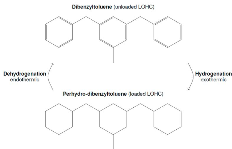
**Figure 1.** Chemical structures of the LOHC system perhydro-dibenzyltoluene/dibenzyltoluene.
