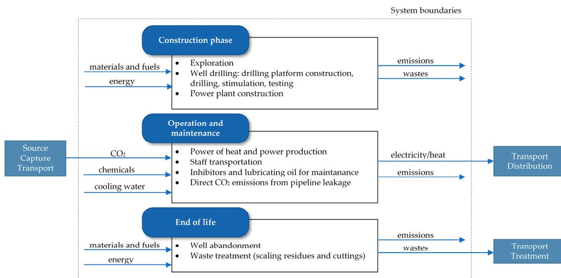
**Figure 1.** sCO<sub>2</sub>-EGS plant life phases with system boundaries.
