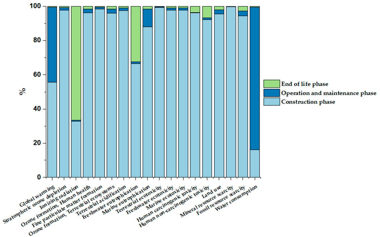
Figure 2. LCA results for Case 1 with exergy allocation for electricity production, ReCiPe 2016, midpoint (H), and characterization.
