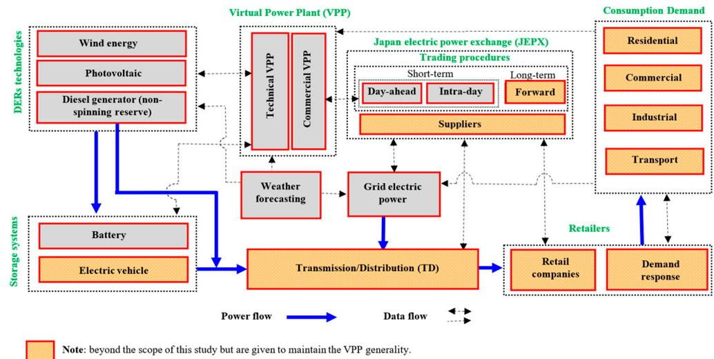
**Figure 1.** Virtual power plant framework and its interaction with the power market and network.
