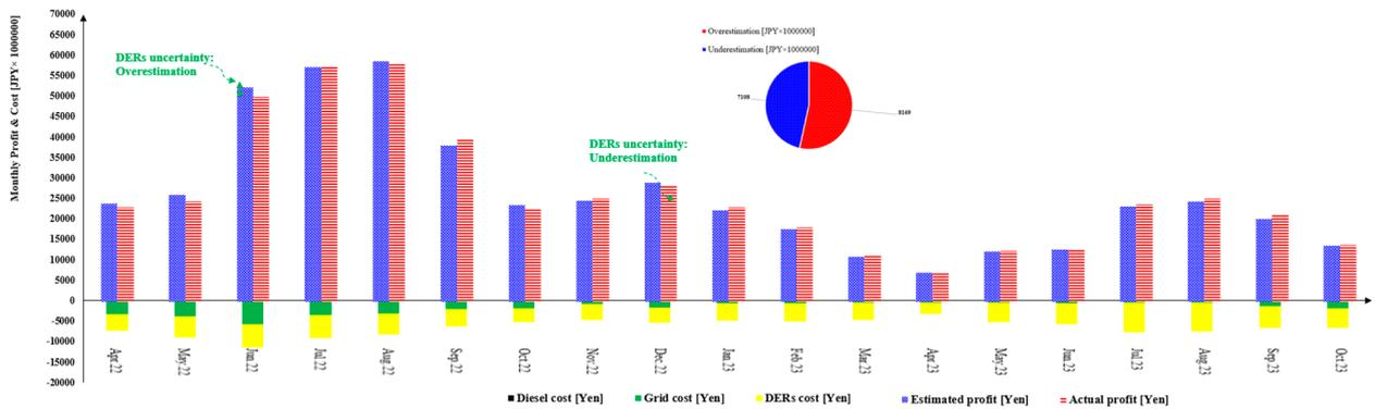
Figure 5. Monthly power generation costs plus expected and actual profit of the VPP system.
