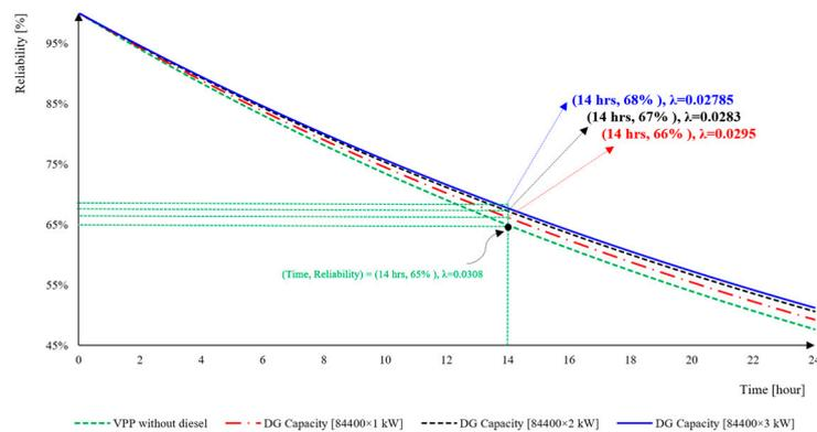
Figure 6. Reliability curves for the VPP system under three different DG capacities.
