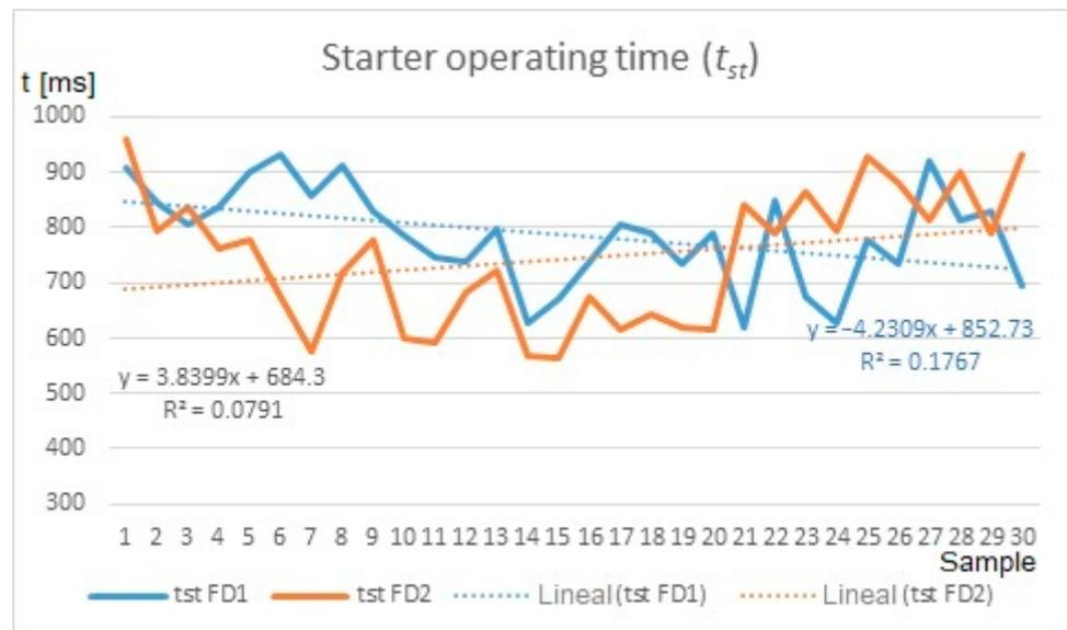
Figure 7. Starter operating time for two measurement series.
