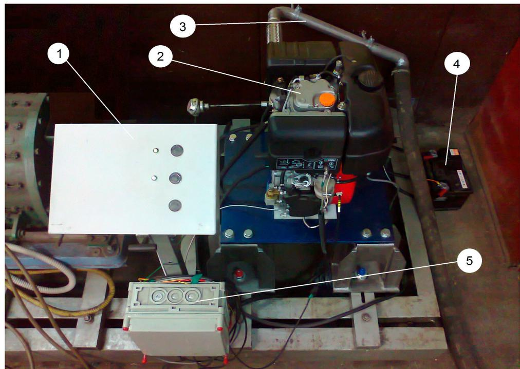
**Figure 1.** View of the research stand: 1—control panel, 2—research engine, 3—exhaust gas discharge system, 4—starting battery, 5—connection of measurement signals [78].
