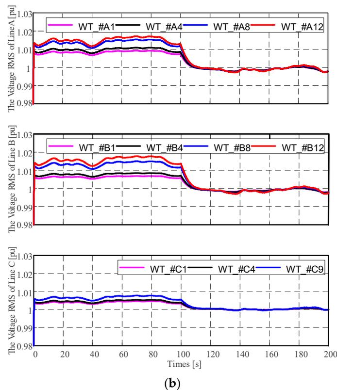
**Figure 5.** Terminal voltage of wind turbines at each feeder in the wind farm: (a) Voltage values on each feeder without relative voltage control; (b) voltage values on each feeder after relative voltage control.
