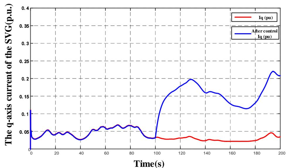
**Figure 6.** Comparison of the power generated by the reactive power compensation device before and after the relative voltage control.
