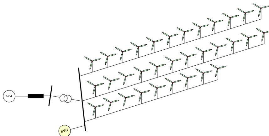
**Figure 1.** Topology of an actual radial wind farm.
