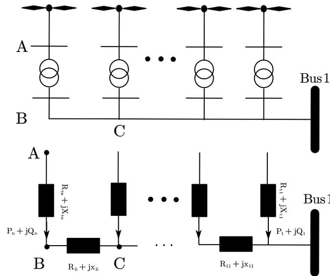
Figure 2. Equivalent model of wind turbines under a certain feeder in a wind farm.
