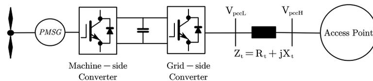
Figure 3. Wind turbine equivalent model and voltage characteristics.
