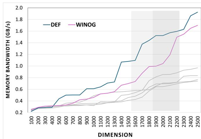
**Figure 6.** Average read/write main memory bandwidth for DEF and WINOG superimposed on the divide-conquer for comparison.
