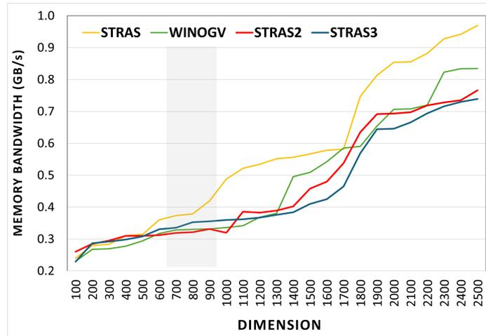
Figure 7. Average read/write main memory bandwidth for the divide-and-conquer group.
