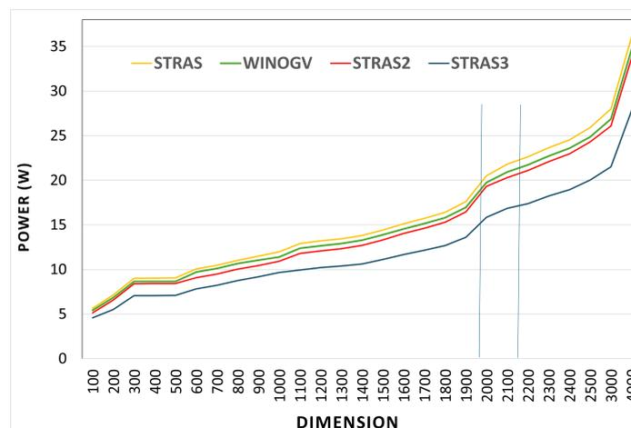
Figure 3. Average power consumption in watts for the divide-and-conquer algorithms.
