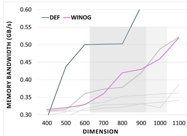
**Figure 9.** Detailed view of the main memory bandwidth showing the probable L2–L3 spillover range.
