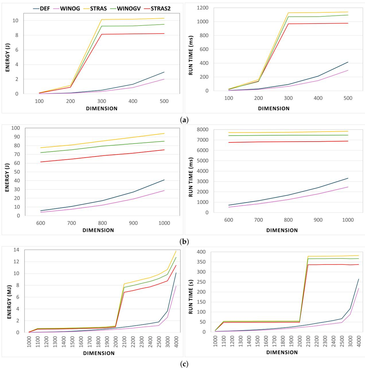
**Figure 2.** Total energy (left) and runtimes (right). The sharp turn at 3000 is due to missing data points. (a) Small matrix size lower range (inside 10 J). (b) Small matrix size upper range (inside 100 J). (c) Large matrices (up to 14K joules, likely DRAM).
