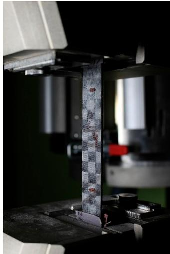
Figure 5. Measurement of tensile properties of the composite sample using the LabTest 6.200.
