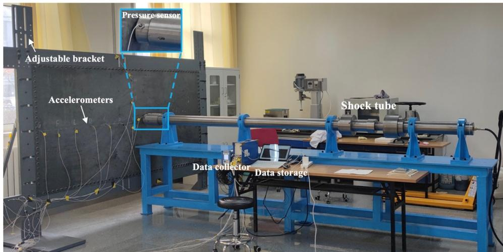
(a) Physical picture of the test device
